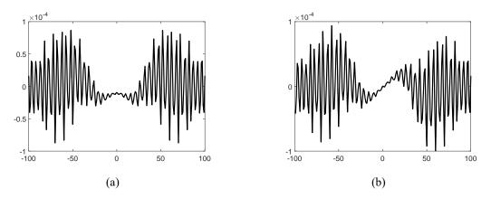
Fig. 6 Comparison of  $u_n(200)$  with different boundary atoms: (a) boundary with same type atoms; (b) boundary with different type atoms. The horizontal axis represents the atomic numbering, and the vertical axis represents the displacement
