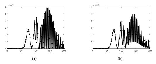
Fig. 7 Energy decay rate for MBC1: solid curve for numerically calculated  $-\dot{E}(t)$  and circle for (a)  $\sqrt{2\gamma/(1+\gamma)}[(u_{-2N} - u_{-2N+1})^2 + (u_{2N-1} - u_{2N})^2]$  (boundary with the same type atoms); (b)  $\sqrt{2\gamma/(1+\gamma)}[(u_{-2N+1} - u_{-2N+2})^2 + (u_{2N-1} - u_{2N})^2]$  (boundary with the different type atoms). The horizontal axis represents time, and the vertical axis represents the rate
