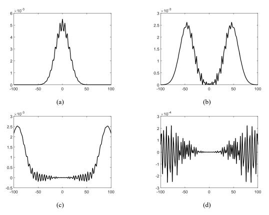
Fig. 4 Displacements with same boundary: (a)  $u_n(0)$ ; (b)  $u_n(40)$ ; (c)  $u_n(80)$ ; (d)  $u_n(120)$ . The horizontal axis represents the atomic numbering, and the vertical axis represents the displacement
