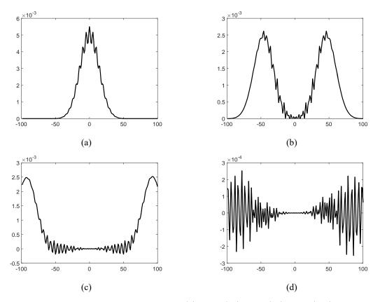
Fig. 5 Displacements with different boundaries: (a)  $u_n(0)$ ; (b)  $u_n(40)$ ; (c)  $u_n(80)$ ; (d)  $u_n(120)$ . The horizontal axis represents the atomic numbering, and the vertical axis represents the displacement
