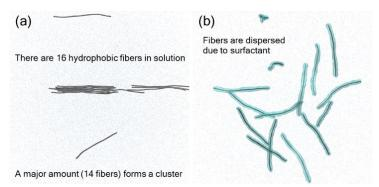
Fig. 3 Schematic drawings of (a) CNTs agglomerates and (b) dispersed CNTs by surfactants. CNTs are represented by chains in gray, water is represented by small dots in light blue and wrapping surfactants are represented by cyan bubbles
