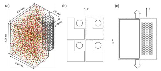
Fig. 5 (a) Snapshots of a single-walled CNT-embedded L-shaped C-S-H. (b) Periodic boundary condition scheme showing repeating images at x and y axis. Tensile tests are performed. (c) Tensile test performed along the longitudinal direction (z axis)
