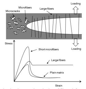
Fig. 1 Schematic diagram showing the general mechanism of fiber reinforcement in cement composite. Gray color indicates solid and white indicates void
