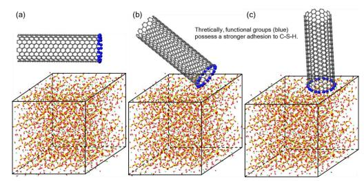
Fig. 2 Schematic drawings of interaction between functionalized CNTs and cement hydrates (C-S-H). Black frame outlines C-S-H gel, where calcium, silicon, hydrogen and oxygen atoms are in green, yellow, white and red respectively. CNT is in gray and representative functional groups are in blue. (a) A single-walled CNT aligns parallel to C-S-H surface. (b) Due to strong adhesion between functional groups (in blue) and C-S-H, the CNT inclines. (c) The CNT chooses a favorable adhesion site
