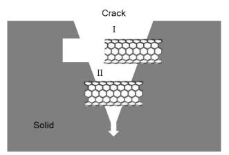
Fig. 4 Schematic diagram of CNTs connecting C-S-H particles, reproduced from (Nadiv *et al.* 2016). Type I represents fracture pulling out, type II represents bridging effect
