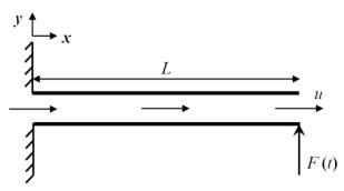
Fig. 1 The simple model of a pipe conveying fluid under electromagnetic damper force
