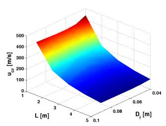
Fig. 2 The effects of the L and  $D_i$  on the critical velocity assuming constant thickness
