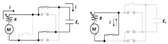
(a) Electric circuit of the electromagnetic damper in regeneration mode when  $\dot{y}(x_F,t) > 0$  (b) Electric circuit of the electromagnetic damper in dissipation mode
