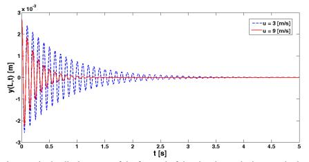
Fig. 3 The decrease in the displacement of the free end of the pipe due to the increase in the fluid flow velocity
