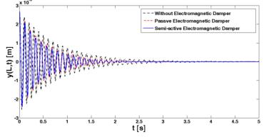
Fig. 7 The vibration of the free end of the pipe with and without electromagnetic damper
