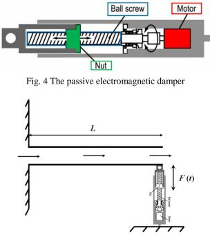
Fig. 5 The electromagnetic damper force at the free end of the pipe
