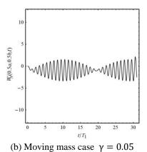
Fig. 5 Thin square plate, 30 moving masses,  $\lambda = 0.5$ ,  $\alpha = 1.0$ : time history of  $W_N$  at the center of the plate
