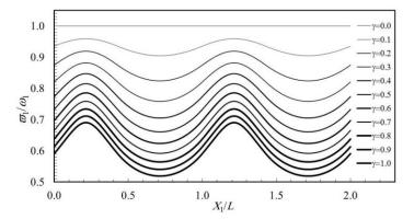
Fig. 6 Thin square plate,  $\lambda = 0.7$ : variation of the fundamental frequency of the plate with the position  $X_1$  of the first attached mass, at varying value of the nondimensional mass  $\gamma$
