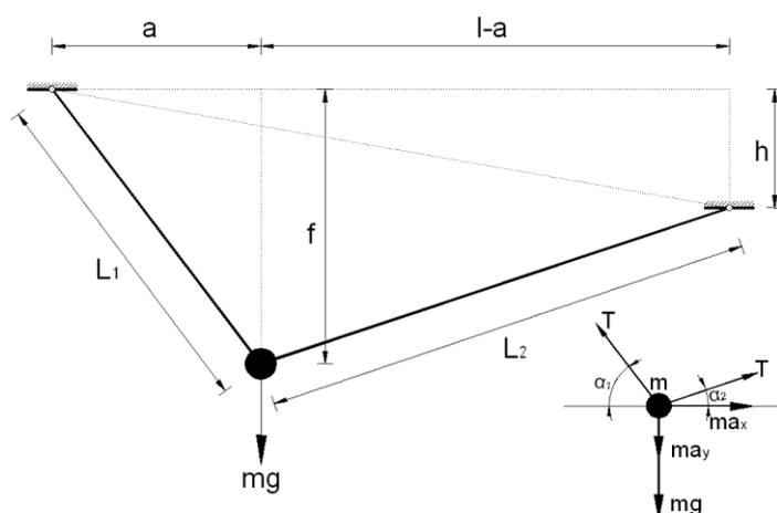
Fig. 1 Sliding mass on the cable and dynamic equilibrium of the sliding mass
