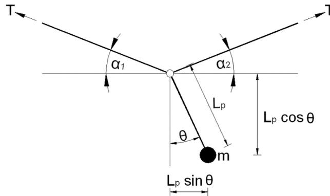
Fig. 3 Coordinates describing pendulum sliding along the rope/cable
