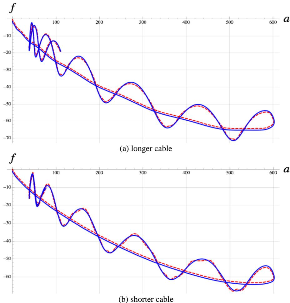
Fig. 8 Mass path in time, position on the cable (dashed red) and pendulum mass (solid blue)
