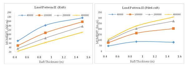
Fig. 10 Variations of maximum moment with raft thickness for raft and piled raft for load pattern-II
