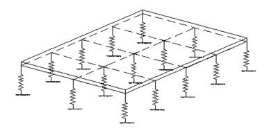
Fig. 1 Structural idealization with raft and supporting soil
