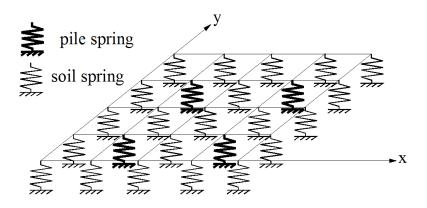
Fig. 2 Structural idealization for piled raft and supporting soil
