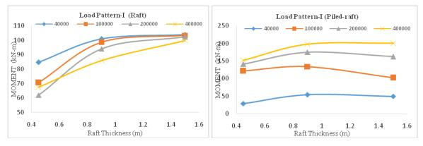
Fig. 8 Variation in maximum moment with raft thickness in raft and piled raft for load pattern-I
