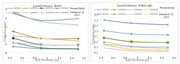
Fig. 7 Variation in maximum deflection in raft and piled raft with raft thickness for load pattern-I
