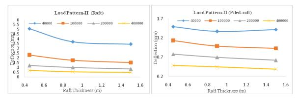
Fig. 9 Variation in maximum deflection with raft thickness in raft and piled raft for load pattern-II
