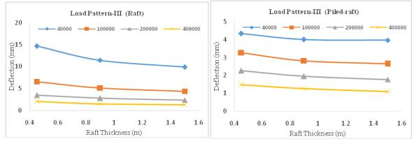
Fig. 11 Variation in maximum deflection with raft thickness in raft and piled raft for load pattern-III
