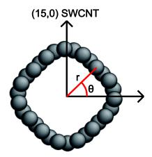
Fig. 1 Top view of the atomic configuration in the axial direction. The (15,0) zigzag SWCNT is radially corrugated with  $\delta r / a = 2.34 \times 10^{-2}$  and n = 4
