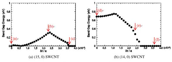
Fig. 3 Change in band gap energy under radial corrugation
