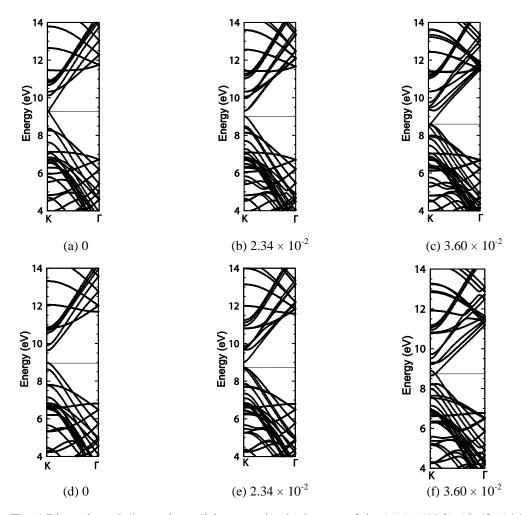
Fig. 4 Dispersion relation under radial corrugation in the case of the (a)-(c) (15,0), (d)-(f) (14,0) zigzag SWCNT. (15,0) SWCNT is the metallic material without any deformation, while (14,0) SWCNT is the semiconducting material without any deformation.
