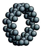
Fig. 2 One period of the radially corrugated atomic configuration of the (15,0) zigzag SWCNT;  $\delta r / a = 2.34 \times 10^{-2}$  and n = 4
