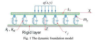
layer  $k_s$ , the viscous damping  $c_f$  and the foundation mass density  $\rho_f$ . Based on the principles of dynamic equilibrium, the mass of the foundation is calculated as several lumped masses  $m_f$  at the top of the elastic springs which connect the elastic springs with the shear layer. The lumped mass  $m_f$  is a parameter that makes the dynamic foundation model significantly different from other models, which are massless ones.
