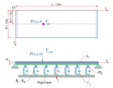
Fig. 5 Model of Mindlin plate on nonlinear dynamic foundation under moving load
