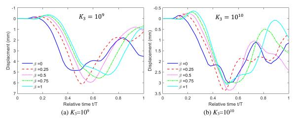
Fig. 9 The vertical displacement of central point of plate for various foundation mass
