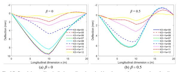
Fig. 8 Deflected shapes of longitudinal centerline when a load is at the center for various values of nonlinear stiffness
