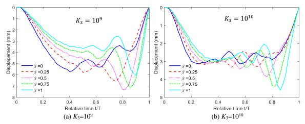
Fig. 10 Vertical displacement under moving load for various foundation mass
