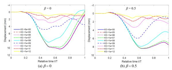
Fig. 6 The displacement of the central point of plate for various values of nonlinear stiffness
