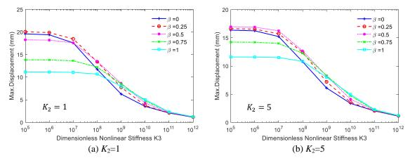
Fig. 15 Effects shear stiffness on max displacement for various nonlinear stiffness and foundation mass where  $K_1 = 50$ ,  $c_f = 100 \text{ Ns/m}^3$
