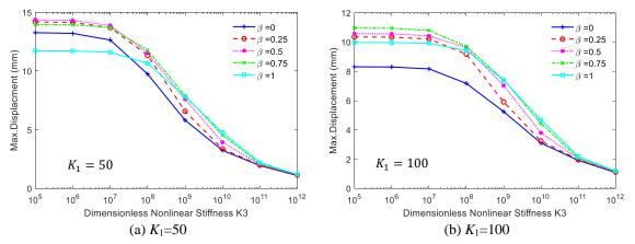
Fig. 14 Effects of linear stiffness on max displacement for various nonlinear stiffness and foundation mass where  $K_2 = 10$ ,  $c_f = 100 \text{ Ns/m}^3$
