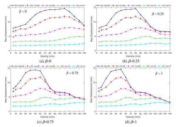
Fig. 12 Effects of the varying load velocities and nonlinear stiffness on max displacement
