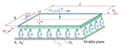
Fig. 3 Model of Mindlin plate on nonlinear dynamic foundation under moving load
