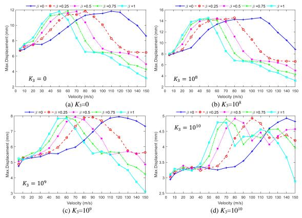
Fig. 13 Effects of the varying load velocities and foundation mass on max displacement
