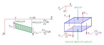
Fig. 2 Dynamic equilibrium on the shear layer: (a) stresses; (b) forces acting
