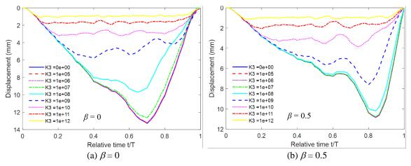
Fig. 7 Vertical displacement under moving load for various values of nonlinear stiffness
