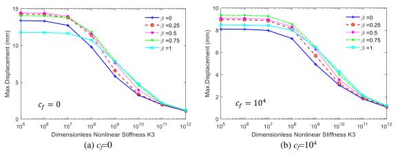
Fig. 16 Effects viscous damping of foundation on max displacement for various nonlinear stiffness and foundation mass where  $K_1 = 50$ ,  $K_2 = 10$
