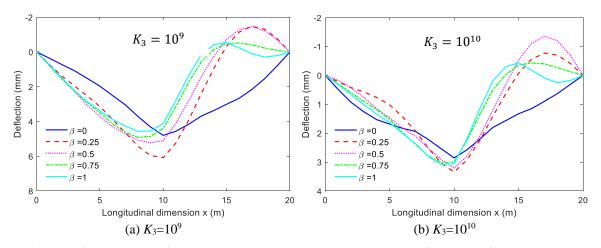
Fig. 11 Deflected shapes of longitudinal centerline when a load is at center for various foundation mass
