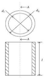
Fig. 1 Hollow shaft
