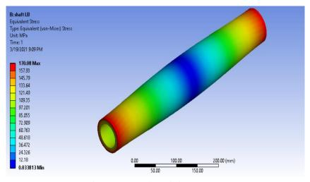
Fig. 7 Stress under twisting moment
