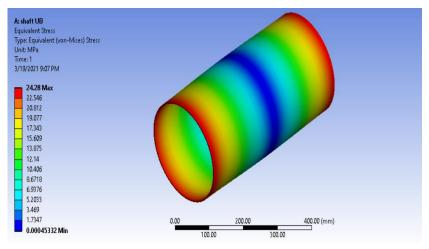
Fig. 4 Stress under twisting moment
