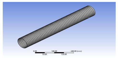
Fig. 8 The meshing of the optimum boundary geometry
