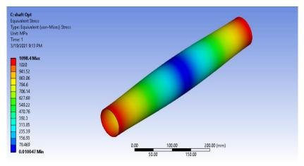
Fig. 10 Stress under twisting moment
