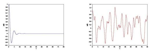
Fig. 10 Response of Duffing oscillator under deterministic load (left) and white noise (right)
