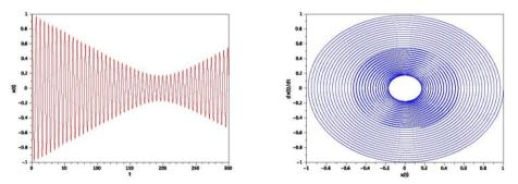
Fig. 9 Computed solution (left) and phase space (right) for Duffing oscillator with numerical values of parameters in (6) chosen as:  $\omega_0 = \delta = \alpha = 1$  and  $\varepsilon = 0.01$
