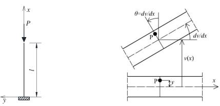
(a) Euler cantilever beam - global configuration(b) Initial and deformed beam axisFig. 1 Classical linearized instability of Euler cantilever beam
