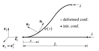
Fig. 2 Nonlinear instability of geometrically exact Euler cantilever beam
