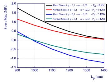
Fig. 9 Effect of plate length of the strengthened beam region Lp on the maximal interfacial stresses for damaged RC cantilever beam strengthening with prestressed laminate plate
