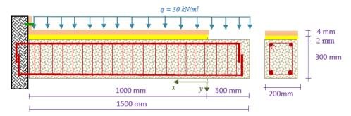
Fig. 3 Geometric characteristics RC damaged cantilever beam strengthening with prestressed composite
