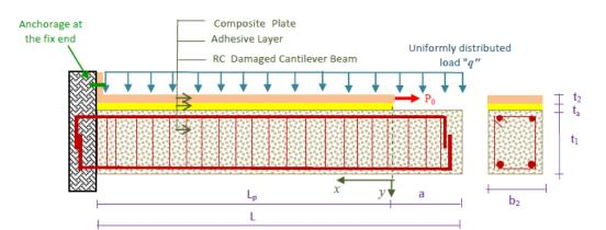
Fig. 1 RC damaged cantilever beam strengthened by a prestressed bonded composite plate
