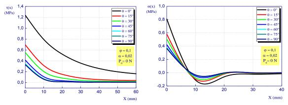
Fig. 11 Effect of various fiber orientations on interfacial stresses for damaged RC cantilever beam strengthening with laminate plate
