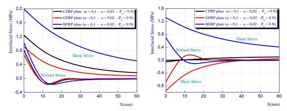
Fig. 7 Effect of plate stiffness on interfacial stresses for damaged RC cantilever beam strengthening with prestressed composite plate
