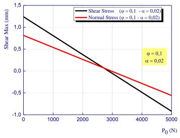
Fig. 6 Effect of prestressing force on interfacial stresses for damaged RC cantilever beam strengthening with prestressed laminate plate
