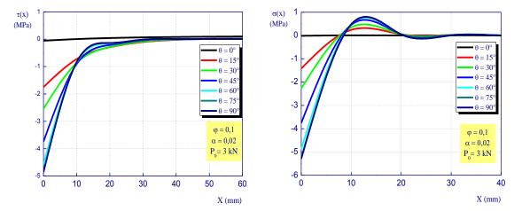
Fig. 12 Effect of various fiber orientations on interfacial stresses for damaged RC cantilever beam strengthening with prestressed laminate plate
