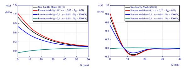
Fig. 4 Variations of interfacial stresses in RC damaged cantilever beam strengthening with prestressed laminate plate: Comparison between the analytical model
