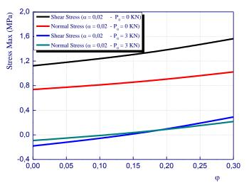
Fig. 8 Effect of damage degree on the maximal interfacial stresses for damaged RC cantilever beam strengthening with prestressed laminate plate
