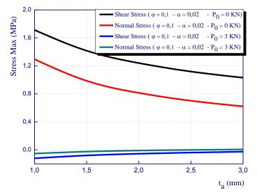
Fig. 10 Effect of the adhesive layer thickness on the maximal interfacial stresses for damaged RC cantilever beam strengthening with prestressed laminate plate
