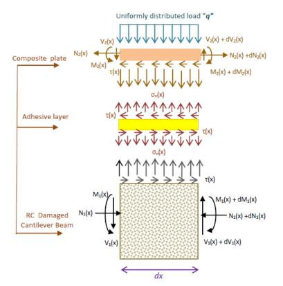
Fig. 2 Forces in differential element of the plated beam
