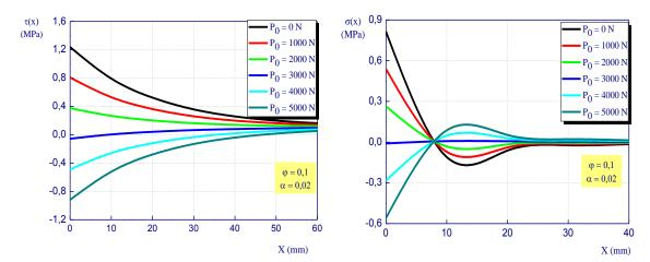
Fig. 5 Adhesive interfacial stresses in RC damaged cantilever beam strengthening with prestressed laminate plate
