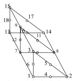
Fig. 2 18 node triangular prism element
