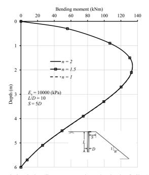
Fig. 8 Variation in bending moment along the depth of pile (S = 5D)
