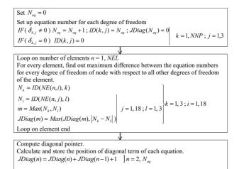
Fig. 3 Algorithm for setup of assembly in skyline storage form
