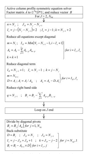
Fig. 4 Algorithm for active column solver
