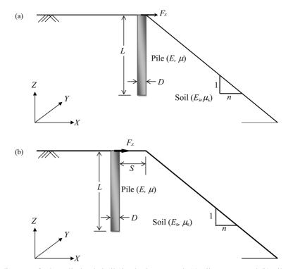
Fig. 1 Schematic diagram of a laterally loaded pile in sloping ground: (a) pile at crest and (b) pile at edge distance, S
