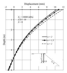
Fig. 5 Displacement pattern along the pile length (S = 0)
