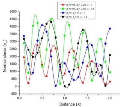
Fig. 13 Variation of normal stress  $\sigma_{33}$  with distance  $x$  (concentrated thermal Source)
