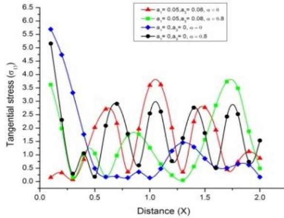
Fig. 5 variation of tangential stress  $\sigma_{31}$  with distance  $x$  (concentrated mechanical force)
