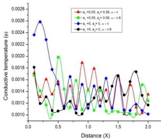
Fig. 9 Variation of conductive temperature  $\phi$  with distance  $x$  (linearly distributed mechanical force)
