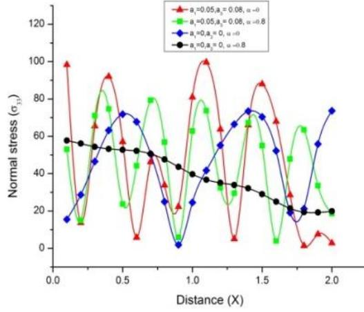
Fig. 18 Variation of normal stress  $\sigma_{33}$  with distance  $x$  (uniformly distributed thermal source)
