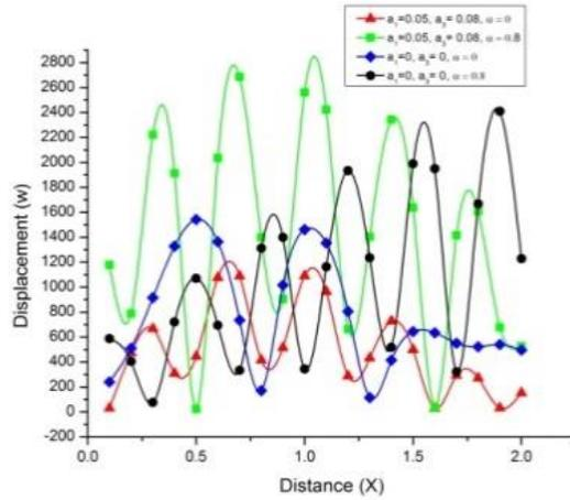
Fig. 12 Variation of normal displacement  $w$  with distance  $x$  (concentrated thermal source)
