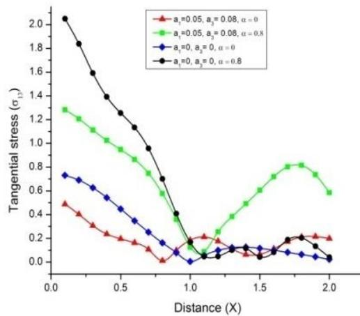
Fig. 10 Variation of tangential stress  $\sigma_{31}$  with distance  $x$  (linearly distributed mechanical force)
