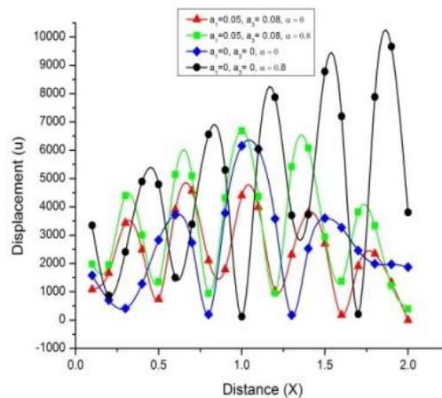
Fig. 11 Variation of tangential displacement  $u$  with distance  $x$  (concentrated thermal source)
