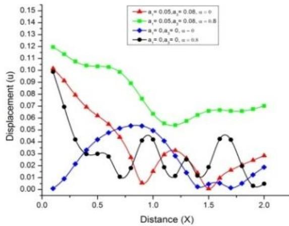
Fig. 6 Variation of tangential displacement  $u$  with distance  $x$  (linearly distributed mechanical force)
