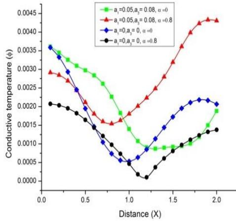
Fig. 19 Variation of conductive temperature  $\phi$  with distance  $x$  (uniformly distributed thermal source)
