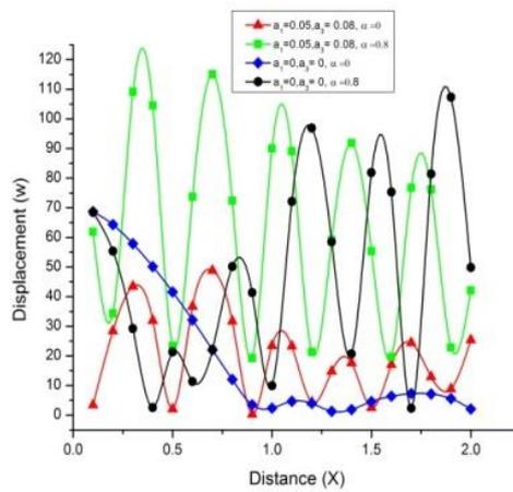
Fig. 17 Variation of normal displacement  $w$  with distance  $x$  (uniformly distributed thermal force)
