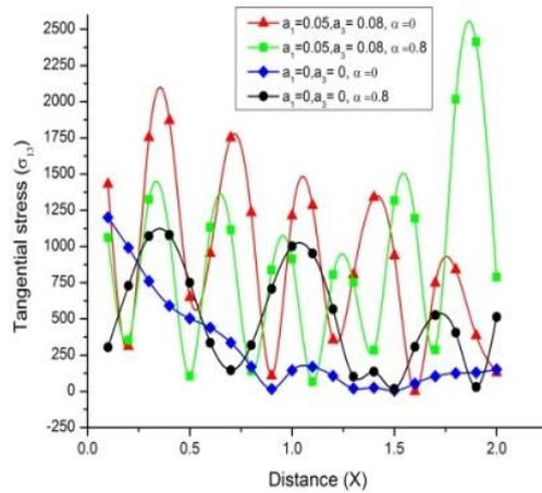
Fig. 20 Variation of tangential stress  $\sigma_{33}$  with distance  $x$  (uniformly distributed thermal source)
