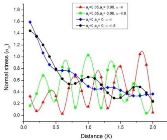
Fig. 3 variation of normal stress  $\sigma_{33}$  with distance  $x$  (concentrated mechanical force)
