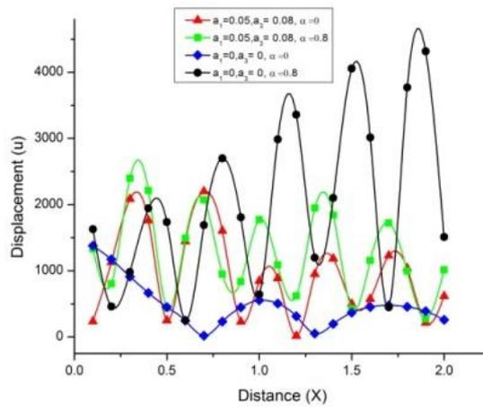
Fig. 16 Variation of tangential displacement  $u$  with distance  $x$  (uniformly distributed thermal force)
