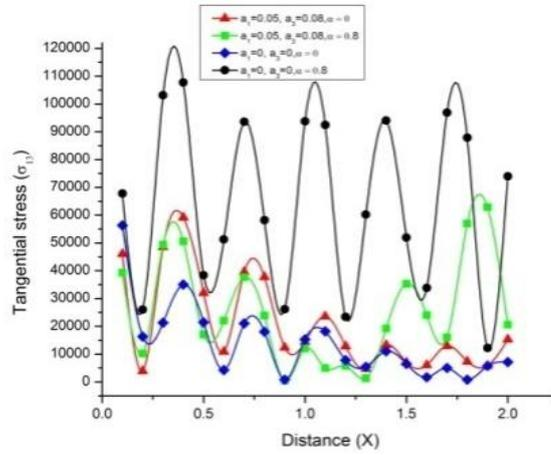
Fig. 15 Variation of tangential stress  $\sigma_{31}$  with distance  $x$  (concentrated thermal source)
