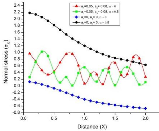
Fig. 8 Variation of normal stress  $\sigma_{33}$  with distance  $x$  (linearly distributed mechanical force)
