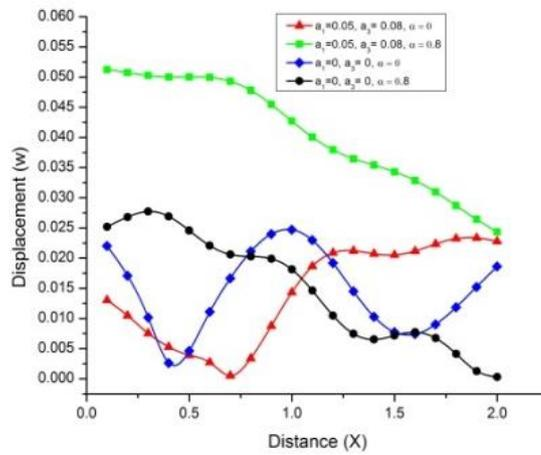
Fig. 7 Variation of normal displacement  $w$  with distance  $x$  (linearly distributed mechanical force)
