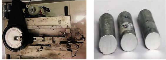
(a) Setup for pin-on-disk wear test
