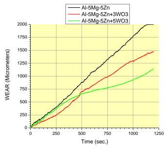
Fig. 5 Dry sliding wear graph of the developed compositions
