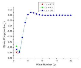
Fig. 4 Variation of stress component  $\sigma_{zz}$  with wave number  $\xi$
