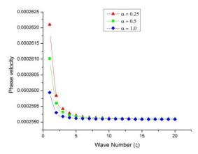
Fig. 1 Variation of phase velocity with wave number  $\xi$
