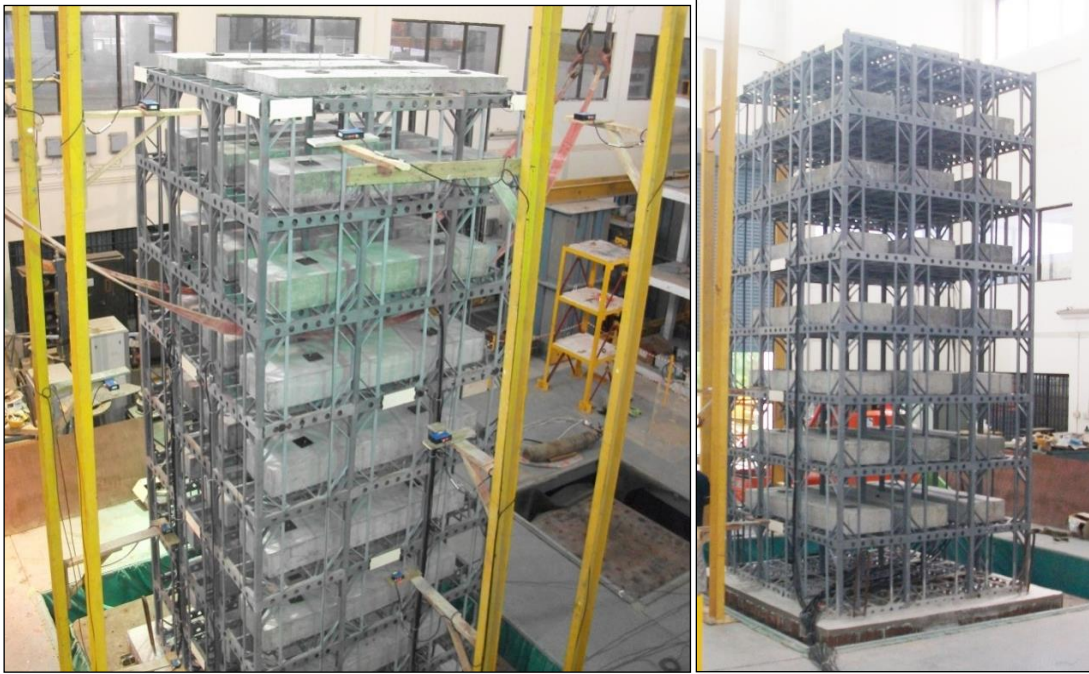
Fig. 4 Shake table testing of a steel building-Case study
