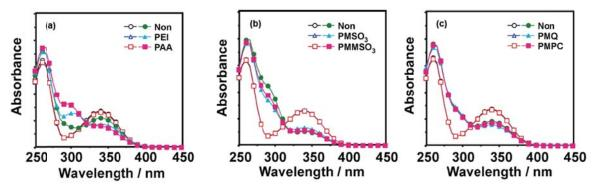
Fig. 5 Effect of the addition of various polymers on the NADH stability. The polymers used were (a) 0.1 wt% PEI and PAA; (b) 1 wt% PMSO<sub>3</sub> and PMMSO<sub>3</sub>; (c) 1 wt% PMQ and PMPC. The storage conditions were (a) pH 7.9 at 25°C for 7 days; (b) pH 7.5 at 25°C for 8 days; (c) pH 7.6 at 37°C for 7 days. The open and solid symbols represent the absorption spectra of NADH in various polymer solutions before and after incubation
