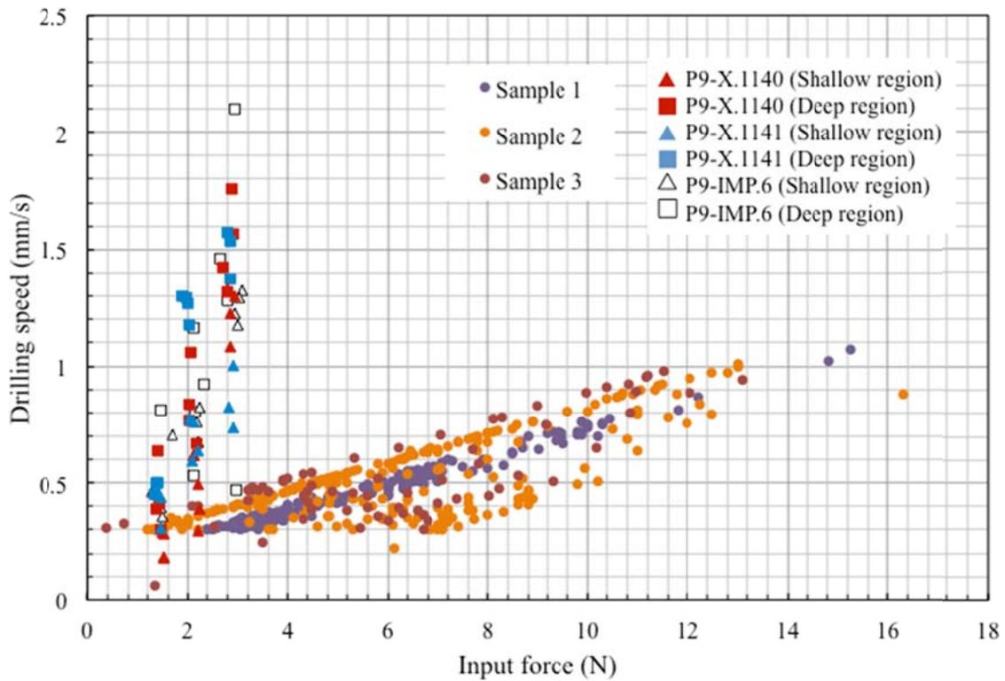
Fig. 7 Results of drilling force and speed on training simulator and polymeric model. The triangular and square markers indicate the results for the polymeric model experiment while the circle marker indicate the three samples evaluated by the clinicians
