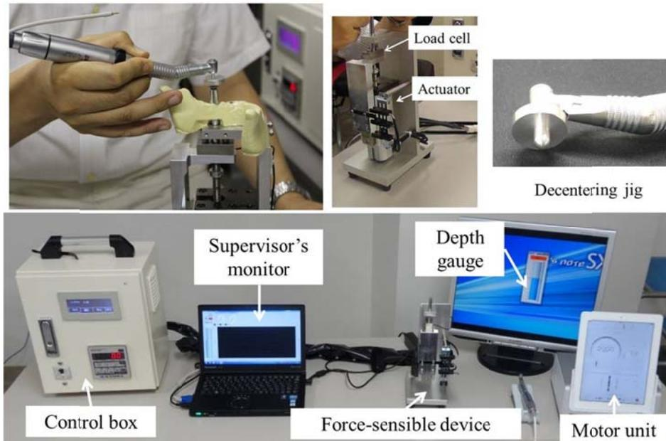
Fig. 1 Developed oral implant surgery simulator. The upper left figure shows a clinician handling the simulator using a decentering jig (upper right) made to be used with this simulator instead of normal drill
