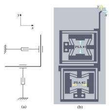
Fig. 9 (a) Scheme of a 2-PP parallel mechanism and (b) a 2-DOF microgripper arm driven by two PSAs (Xu 2012)
