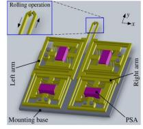
Fig. 10 A two-arm 2-DOF microgripper (Xu 2012)
