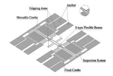
Fig. 4 An electrostatic microgripper design (Hamedi et al. 2012)
