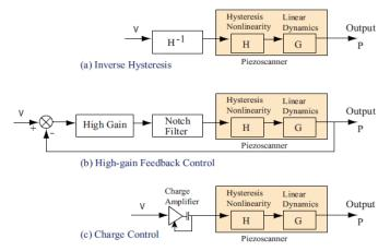
Fig. 15 Three different approaches to linearize hysteresis nonlinearity in piezoscanners (Clayton *et al.* 2009)
