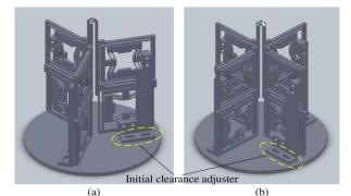
Fig. 11 (a) A three-arm and (b) a four-arm microgrippers (Xu 2012)
