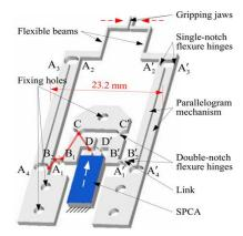
Fig. 8 3-D drawing of the MCM with an SPCA (Wang et al. 2011)
