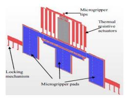
Fig. 13 Active microgripper (Anis et al. 2006)
