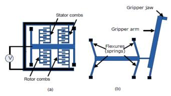
Fig. 2 (a) Voltage applied to actuator combs (b) Gripper arm bent due to force applied by the comb drives (Amjad *et al.* 2008)
