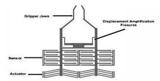
Fig. 5 Schematic diagram of electrothermal microgripper (Ali et al. 2011)
