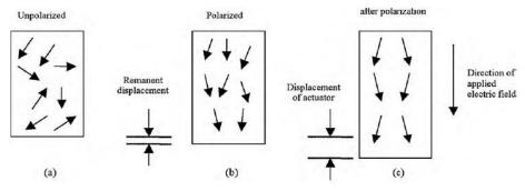
Fig. 6 Polarization process for a piezoelectric actuator (Devasia et al. 2007)
