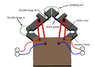
Fig. 14 Conceptual drawing of microgripper (Kyung et al. 2007)
