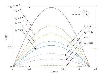
Fig. 4 Radial displacement at the inner and outer surfaces for various values of k3
