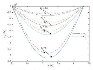
Fig. 6 Radial stress distribution at the inner and outer surfaces for various values of  $k_3$
