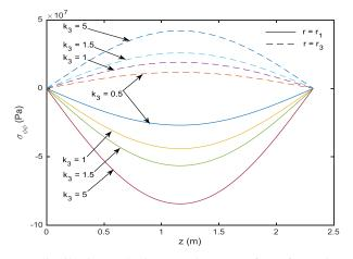
Fig. 7 Hoop stress distribution at the inner and outer surfaces for various values of  $k_3$
