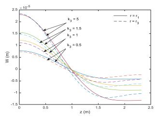
Fig. 5 Axial displacement at the inner and outer surfaces for various values of k3
