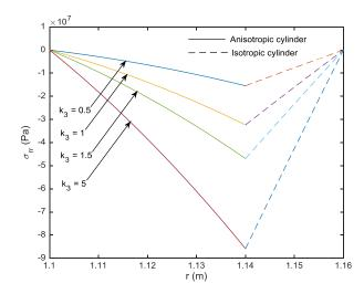
Fig. 10 Radial stress distribution in r-direction for z = L/2
