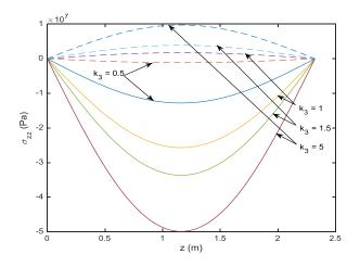
Fig. 8 Axial stress distribution at the inner and outer surfaces for various values of  $k_3$
