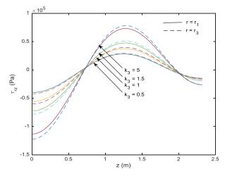
Fig. 9 Shear stress distribution at the inner and outer surfaces for various values of  $k_3$
