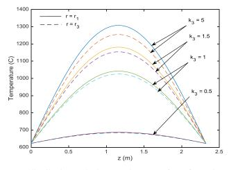
Fig. 2 Temperature distribution at the inner and outer surfaces for various values of k<sub>3</sub>
