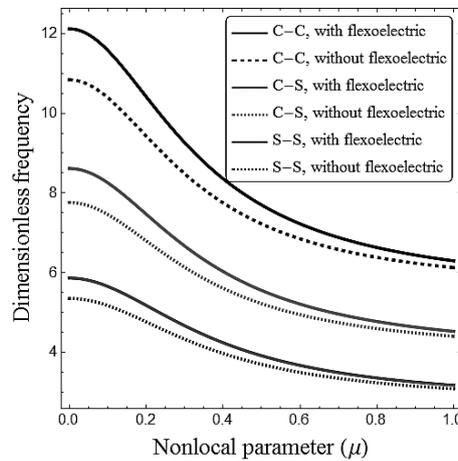
Fig. 5 Flexoelectric and nonlocal impacts on vibrational frequency of nonlocal piezoelectric beams for different boundary conditions ( $L/h = 20, \Delta T = 200\text{K}$ )
