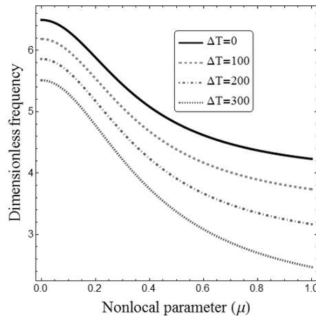
Fig. 3 Nonlocal and temperature variation impacts on vibrational frequency of flexoelectric nano-size beam ( $L/h = 20$ )
