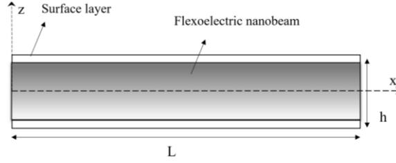
Fig. 1 Geometry of flexoelectric nano-size beam with surface layers
