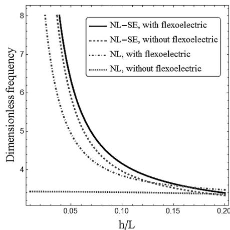
Fig. 4 Surface and flexoelectric impacts on vibrational frequency variation with respect to thickness ( $\mu = 0.1$ )
