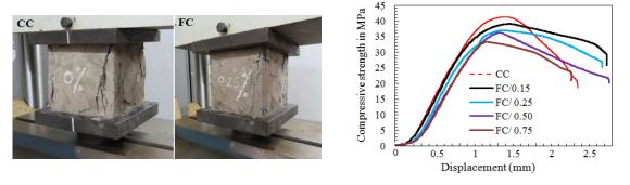
Fig. 4 Compressive strength test (a) Failure pattern; (b) Variation of strength with respect to fiber dosage
