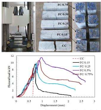
Fig. 6 Flexural strength test (a) test set-up, failure pattern and fiber distributions; (b) Variation of strength with respect to fiber dosage
