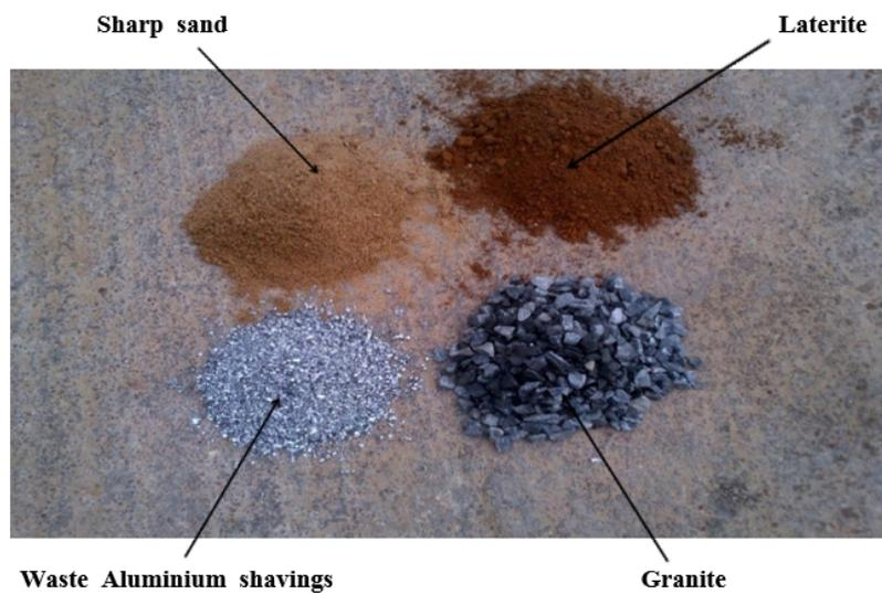
Fig. 4 Aggregates and waste aluminum shavings
