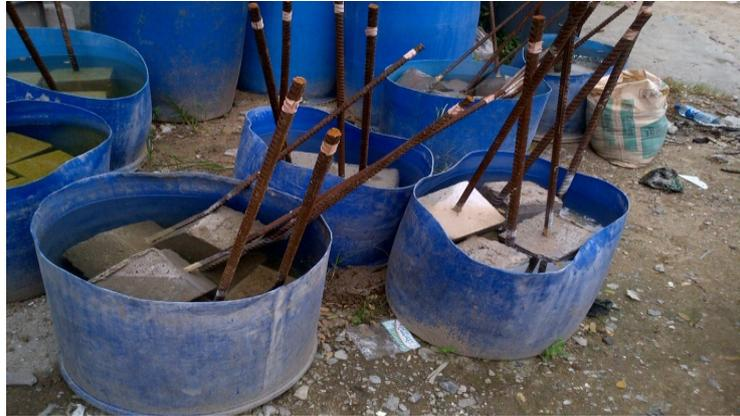
Fig. 5 Curing of RILEM pullout specimens
