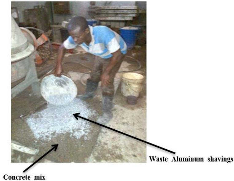
Fig. 2 Mixing of concrete with waste aluminum shavings
