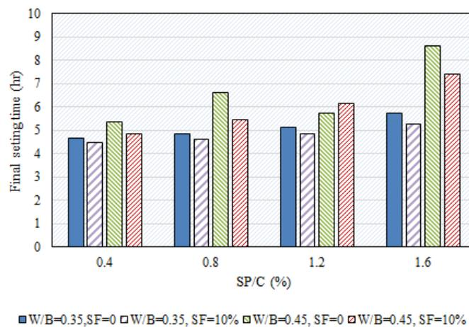
Fig. 4 Effect of superplasticizer dosage on final setting time of pastes
