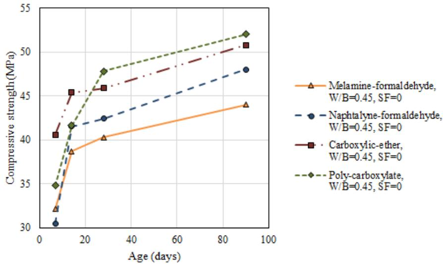
Fig. 15 Variation of compressive strength with time in mixes with W/B=0.45 and SF/C=0%
