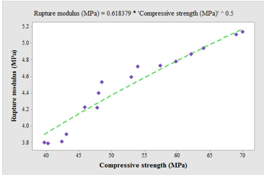
Fig. 21 Correlation between modulus of rupture and compressive strength
