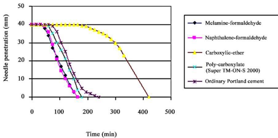
Fig. 12 Setting time of paste with SF=10%
