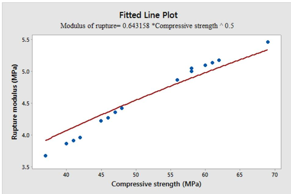
Fig. 9 28-day rupture modulus versus 28-day compressive strength
