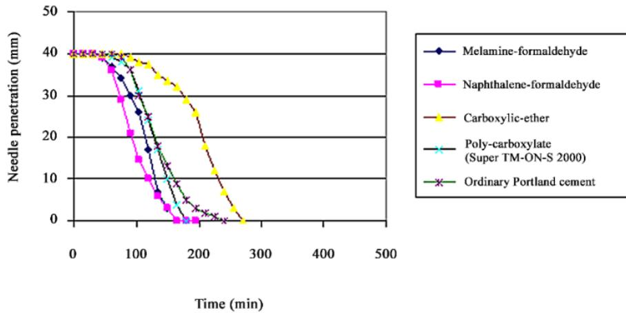
Fig. 11 Setting time of paste with SF=0
