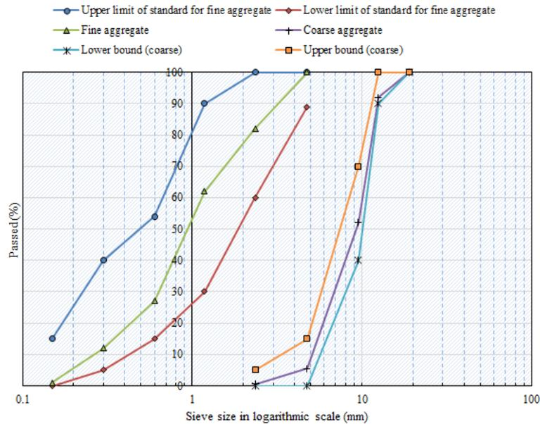
Fig. 1 Grading of coarse and fine aggregates of series A
