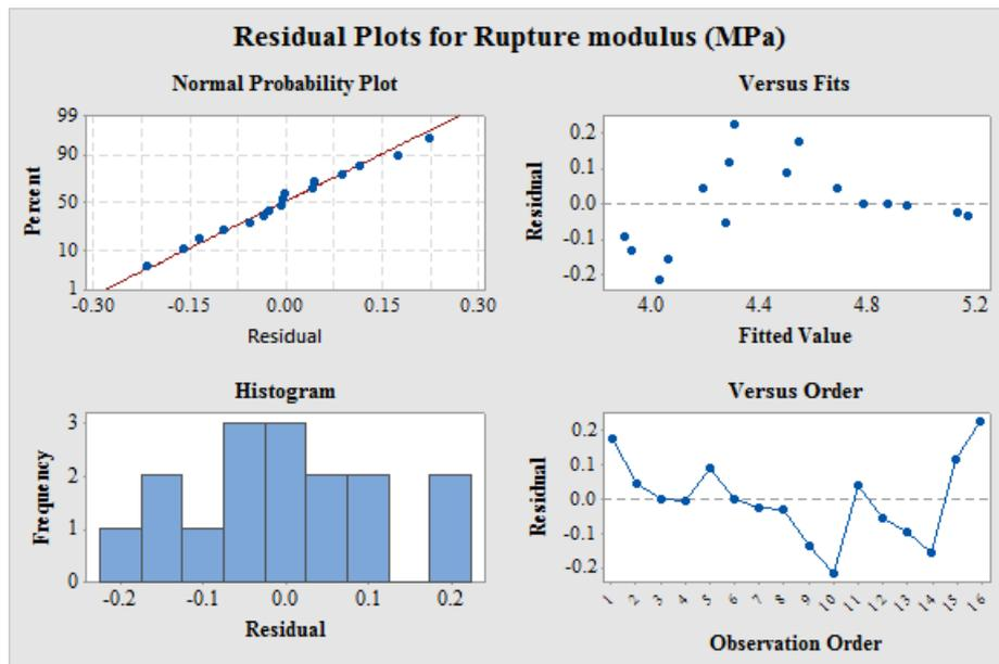
Fig. 22 Residual plots for the fitted curve of rupture modulus
