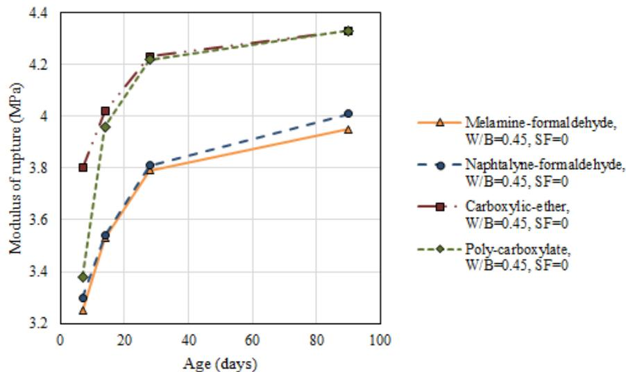
Fig. 18 Variation of rupture modulus with time in mixes with W/B=0.45 and SF/C=0%
