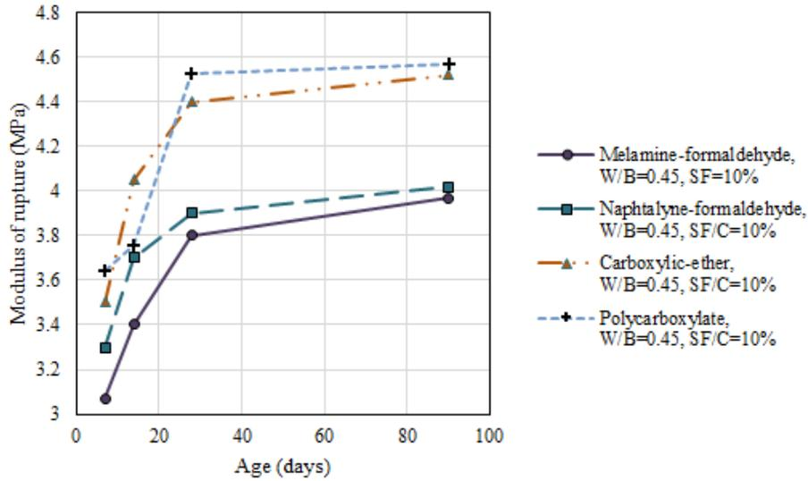
Fig. 19 Variation of rupture modulus with time in mixes with W/B=0.45 and SF/C=10%
