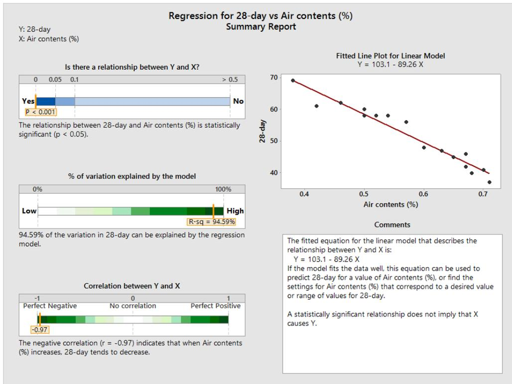
Fig. 7 The correlation between the air contents of the samples of series A and their 28-day compressive strength
