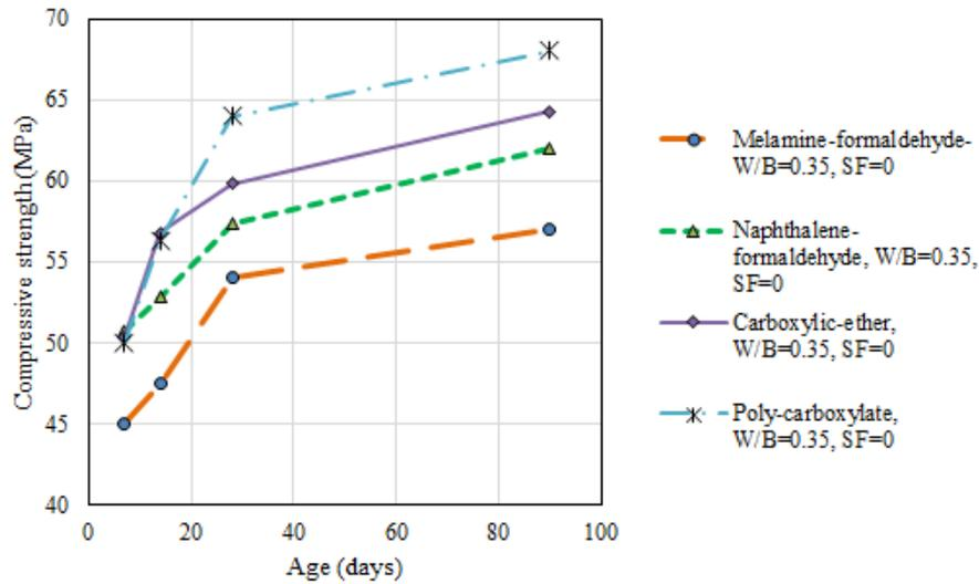
Fig. 13 Variation of compressive strength with time in mixes with W/B=0.35 and SF=0
