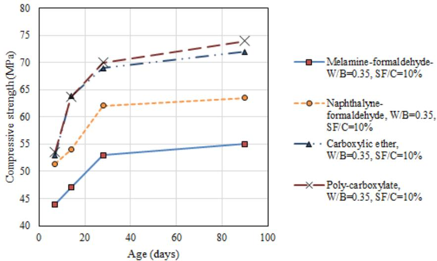
Fig. 14 Variation of compressive strength with time in mixes with W/B=0.35 and SF/C=10%
