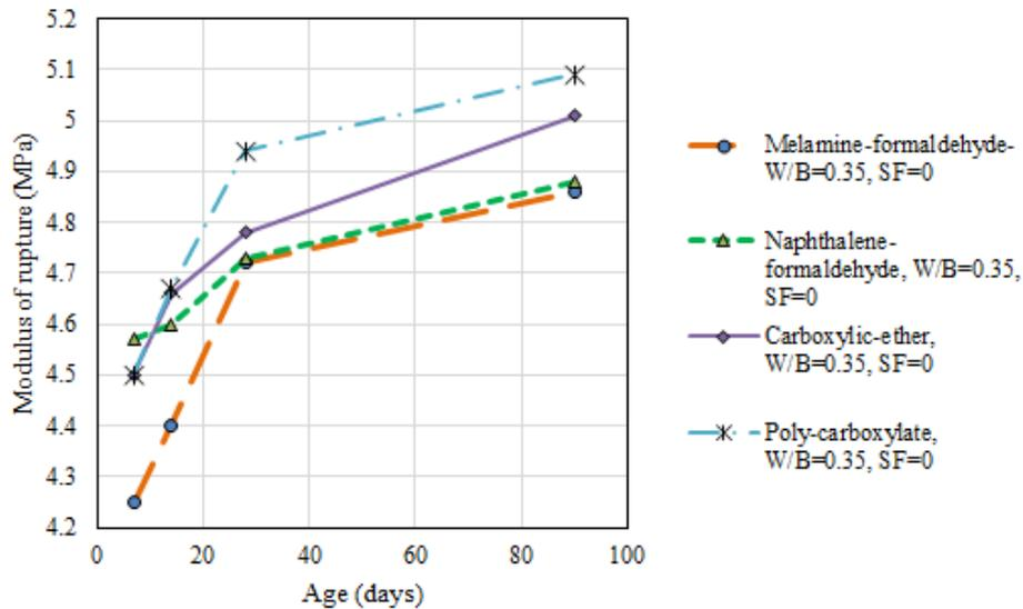
Fig. 17 Variation of rupture modulus with time in mixes with W/B=0.35 and SF/C=0%
