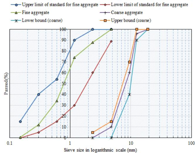
Fig. 2 Grading of coarse and fine aggregates of series B
