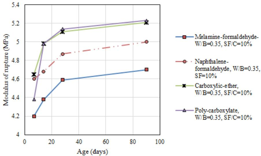
Fig. 20 Variation of rupture modulus with time in mixes with W/B=0.35 and SF/C=10%
