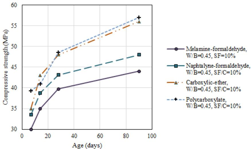
Fig. 16 Variation of compressive strength with time in mixes with W/B=0.45 and SF/C=10%
