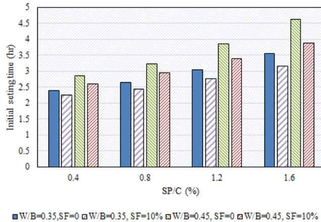
Fig. 3 Effect of superplasticizer dosage on initial setting time of pastes
