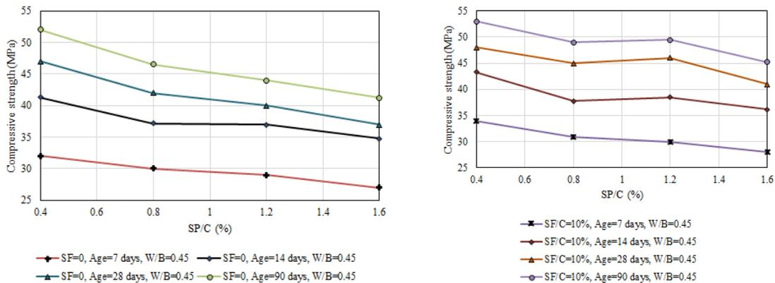
Fig. 8 The effect of SP dosage on compressive strength of mixes with W/B=0.45, SF=0 (left) and SF/C=10% (Right)
