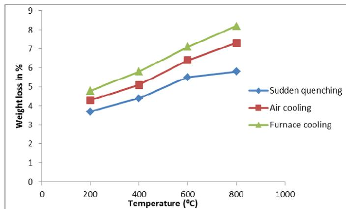
Fig. 3 Variation of loss in weight with temperature
