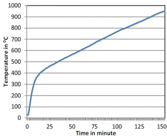
Fig. 2 Time Vs. Temperature build up curve for the furnace
