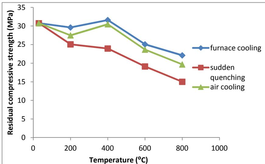
Fig. 6 Residual compressive strength of concrete with PP fibers
