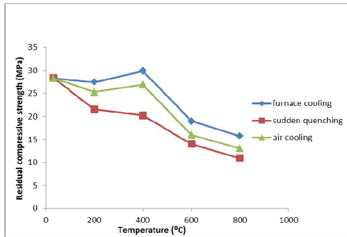
Fig. 5 Residual compressive strength of normal concrete
