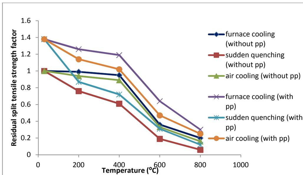
Fig. 8 Residual split tensile strength factor of concrete with and without polypropylene fibres
