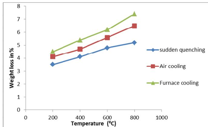
Fig. 4 Weight loss of concrete with polypropylene fibres
