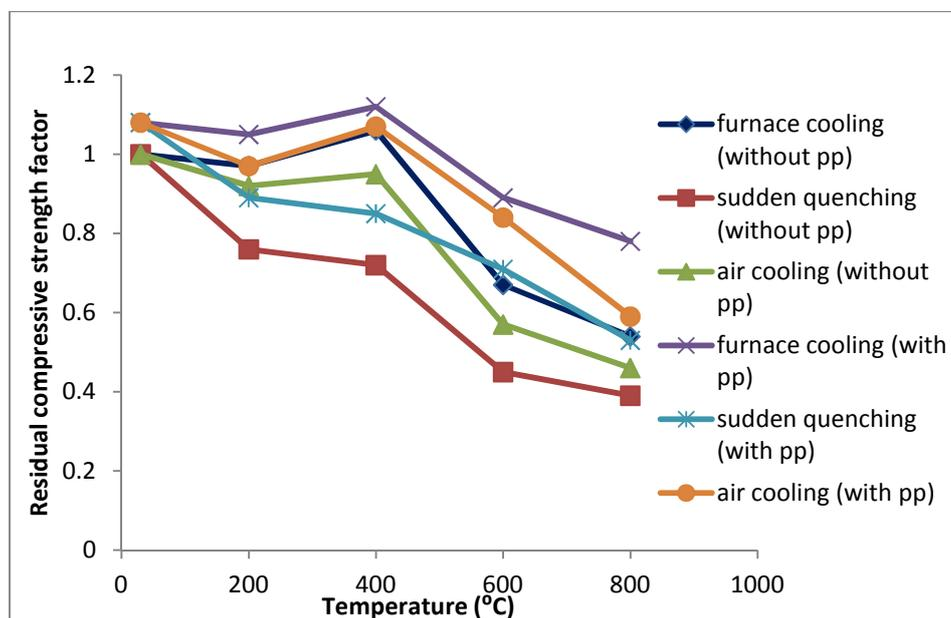
Fig. 7 Variation in residual strengths of concretes, with temperature under different cooling regimes
