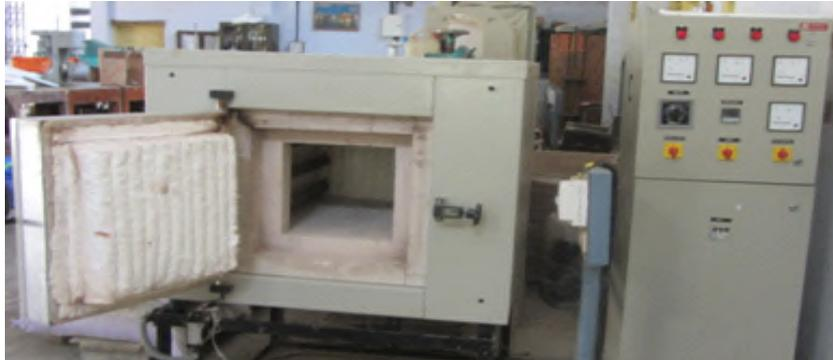
Fig. 1 Programmable electric furnace
