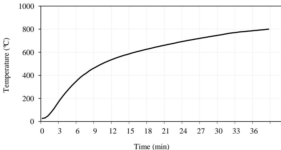
Fig. 2 Maximum rate of heating of furnace with no charge
