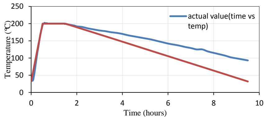
Fig.6 Furnace performance at 200°C with 40kg charge
