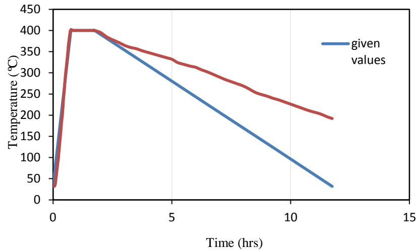
Fig. 7 Furnace performance at 400°C with 40kg charge
