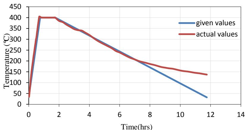
Fig. 4 Furnace performance at 400°C and no charge
