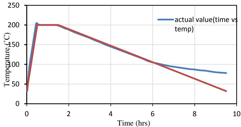
Fig. 3 Furnace performance at 200°C and no charge
