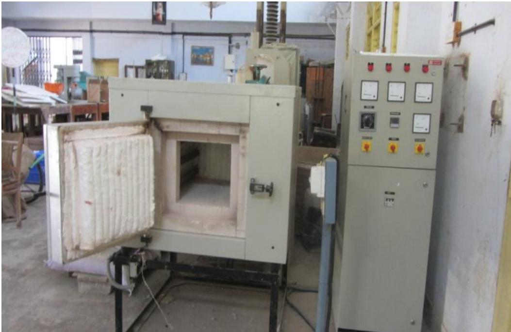
Fig. 1 Programmable electric furnace
