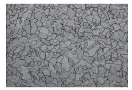
Fig. 1 Microstructure of experimental steel annealed in received condition (Normalized)
