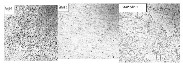
Fig. 2 Optical microstructure of steel annealed at  $750^{\circ}C$
