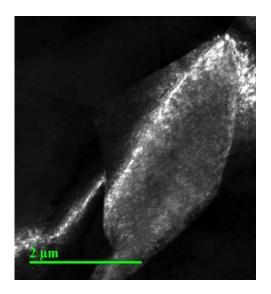
Fig. 11 Dark field photograph of martensite
