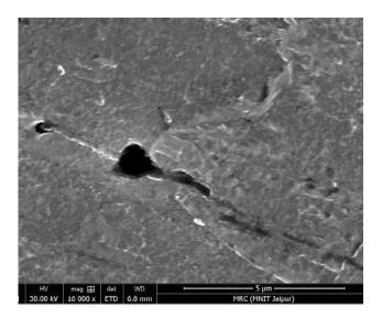
Fig. 8 Scanning electron micrograph of steel annealed at  $700^{\circ}C$
