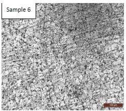
Fig. 6 Optical microstructures of steel annealed at  $675^{\circ}$ C for 4 hrs
