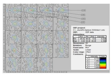
Fig. 16 ODF of steel annealed at  $800^{\circ}C$
