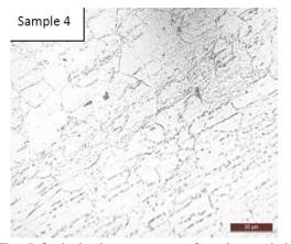
Fig. 5 Optical microstructures of steel annealed at  $675^{\circ}$ C for 1hr
