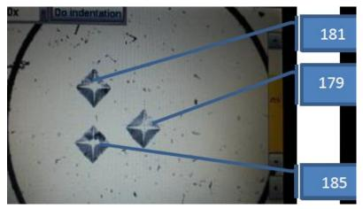
Fig. 7(a) Microhardness results of steel annealed at  $750^{\circ}C$
