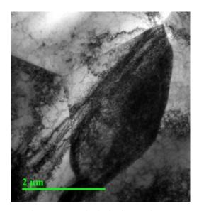
Fig. 10 Martensite in ferrite matrix, BF
