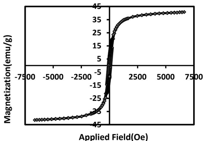
Fig. 6 Magnetization vs. applied magnetic field for of Fe<sub>3</sub>O<sub>4</sub>-PASC nanocomposite
