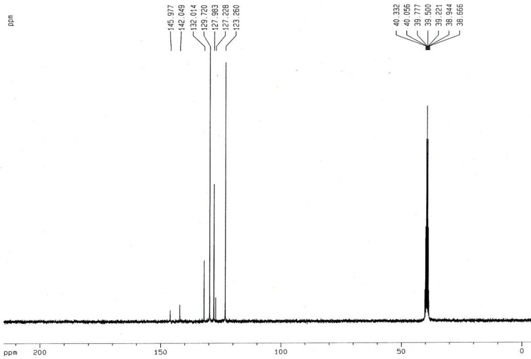
Fig. 2 FT-<sup>13</sup>C NMR of Fe<sub>3</sub>O<sub>4</sub>-PASC nanocomposite
