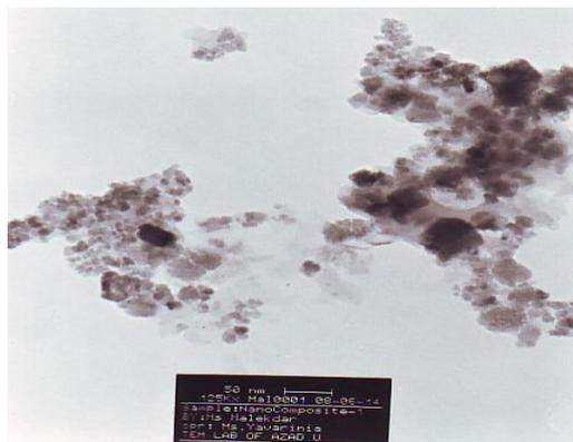
Fig. 4 The TEM photograph Fe<sub>3</sub>O<sub>4</sub>-PASC nanocomposite containing 15% wt nanoparticle
