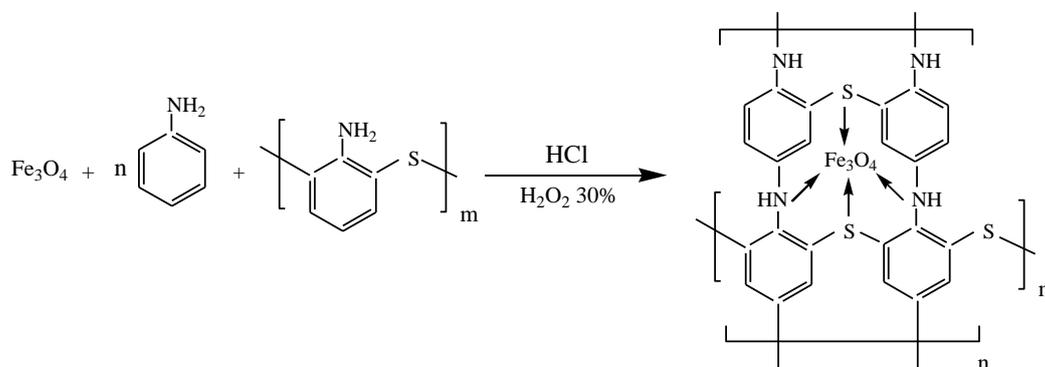
conductivity, flexibility and solubility similar to pure polyaniline, can be obtained. Uniform- sized  $\text{Fe}_3\text{O}_4$ -PASC nanocomposite containing different amount of magnetic nanoparticles has been prepared through modified polymerization.
