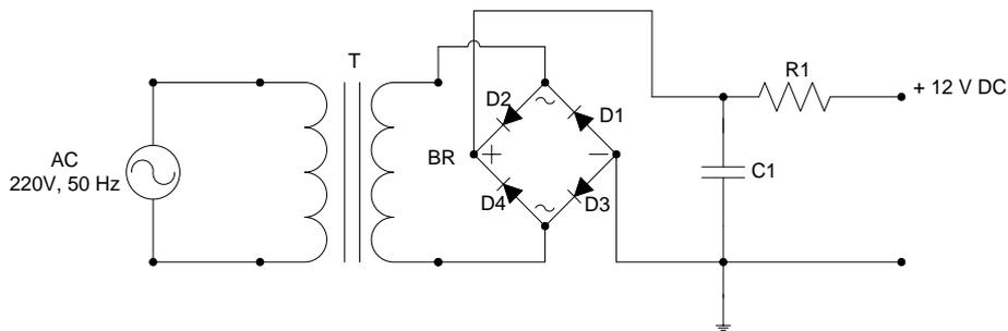
Fig. 1 Realization circuit of a DC Power Supply Circuit
