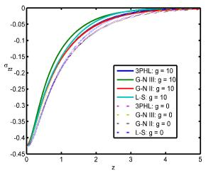
Fig. 11 Variation of stress component  $\sigma_{zz}$  for different theories in the presence and absence the gravitational field
