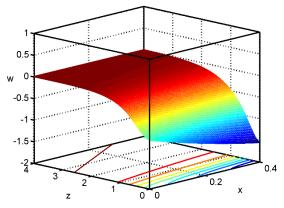
Fig. 13 (3D curve) Distribution of the displacement w versus the distances for 3PHL at  $g=9.8~\rm m\cdot s^{-2}$ ,  $H_0=120~\rm A^{-1}\cdot m^{-1}$
