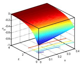
Fig. 15 (3D curve) Distribution of the stress component  $\sigma_{zz}$  versus the distances for 3PHL at  $g=9.8~m.\,s^{-2}$ ,  $H_0=120~A^{-1}\cdot m^{-1}$
