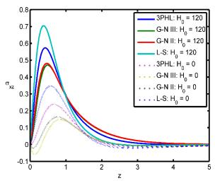
Fig. 8 Variation of stress component  $\sigma_{xz}$  for different theories in the presence and absence the magnetic field
