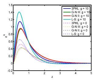
Fig. 12 Variation of stress component  $\sigma_{xz}$  for different theories in the presence and absence the gravitational field
