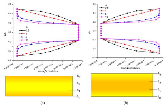
Fig. 2 Variation of Young's modulus across the thickness for 1-1-1 (a) H-Type-A and (b) S-Type-A sandwich FG plate
