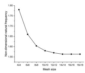
Fig. 5 Convergence study for SSSS H-Type-A sandwich plate (*a/h*=100, *n*=0.5)
