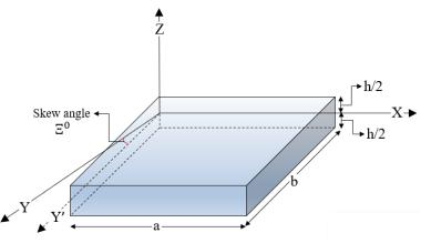
Fig. 1 Geometry of skew sandwich FG plate
