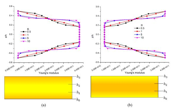
Fig. 4 Variation of Young's modulus across the thickness for 1-1-1 (a) H-Type-S and (b) S-Type-S sandwich FG plate
