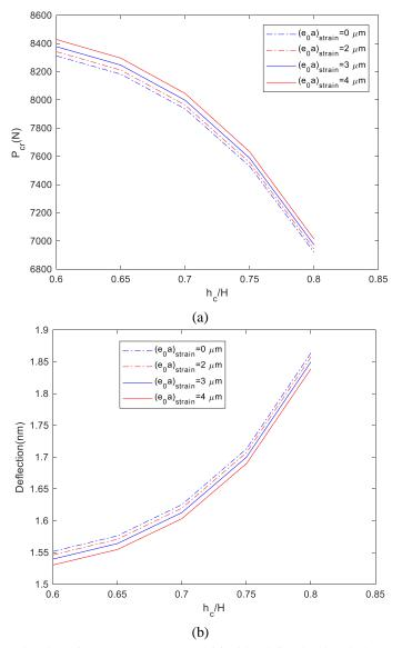
Fig. 2 The effect of nonlocal strain parameter on (a) Critical buckling load and (b) Transverse deflection of sandwich beam
