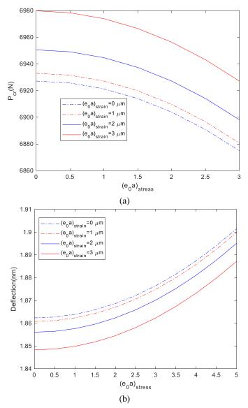
Fig. 4 The effect of nonlocal both stress and strain parameters on (a) Critical buckling load and (b) Transverse deflection of sandwich beamy
