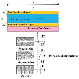
Fig. 1 The schematic view of a sandwich beam with various distributions of porous core and functionally graded top and bottom facesheet layers
