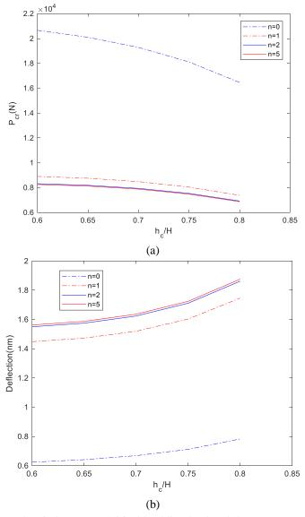
Fig. 5 The effect of power law index on (a) Critical buckling load and (b) Transverse deflection of sandwich beam
