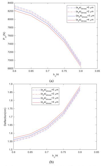
Fig. 3 The effect of nonlocal stress parameter on (a) Critical buckling load and (b) Transverse deflection of sandwich beam
