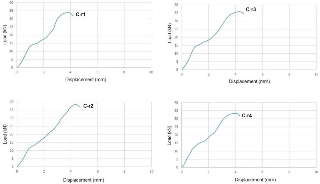
Fig. 9 Load displacement graphs from the pull-out test of cone bolts without the polyamide absorber ring and in the grout mix without the STP additive
