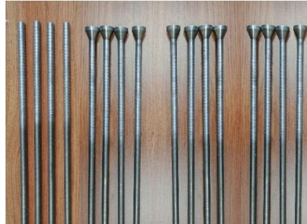
Fig. 3 Rock bolts used in this study
