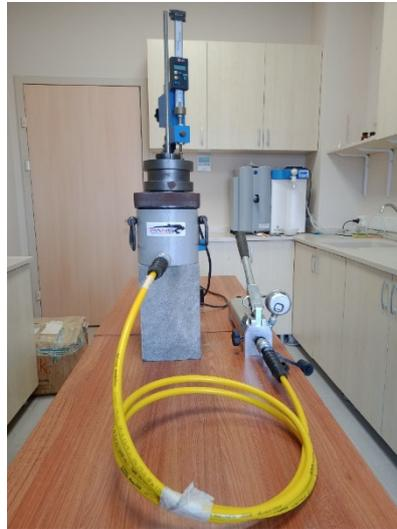
Fig. 7 The pull-out test performed in this study
