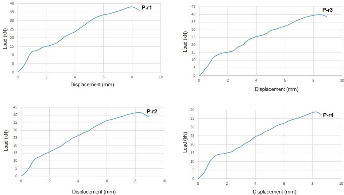
Fig. 11 Load displacement graphs from the pull-out test of cone bolts with the polyamide absorber
