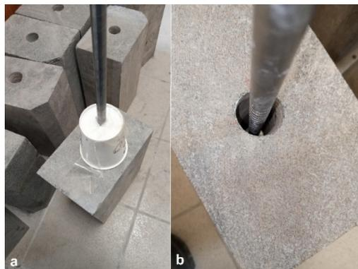
Fig. 4 (a) Use of drilled cup to hold bolts without expanded (cone) end; (b) ability of cone bolts to stand by itself
