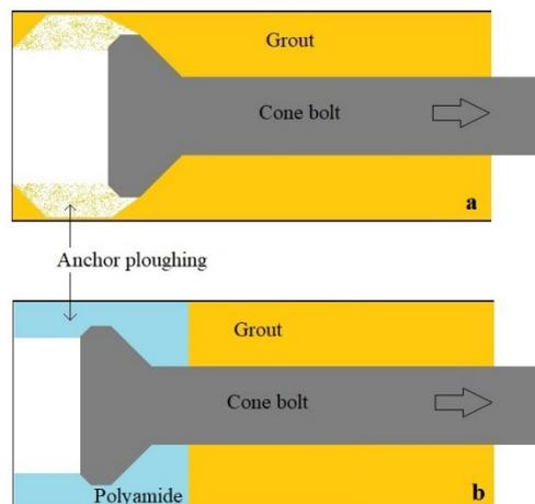
Fig. 1 Anchoring mechanism of the cone part in grout (a) and in the polyamide energy absorber ring (b)
