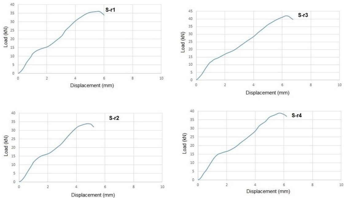
Fig. 10 Load displacement graphs from the pull-out test of cone bolts in the STP added cement grout
