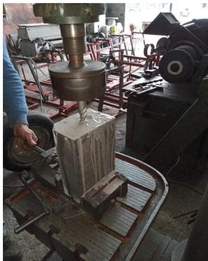
Fig. 2 Drilling rock blocks
