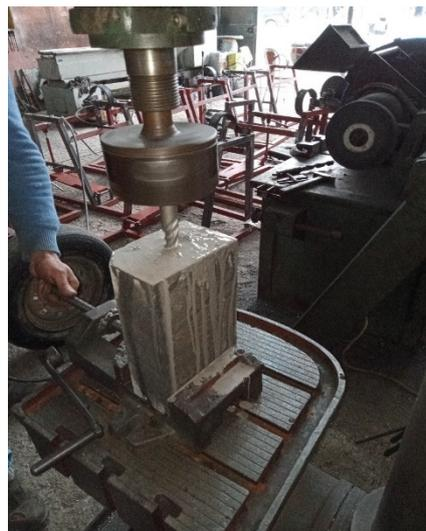
Fig. 2 Drilling rock blocks
