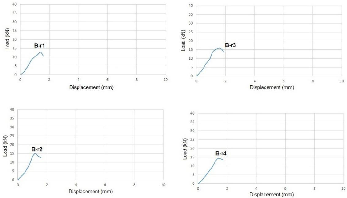
Fig. 8 Load displacement graphs from the pull-out test of bolts without cone ends (r: replicate)
