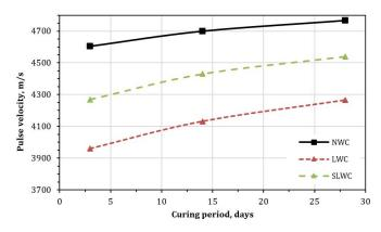
Fig. 5 Pulse velocity development in SLWC and LWC specimens
