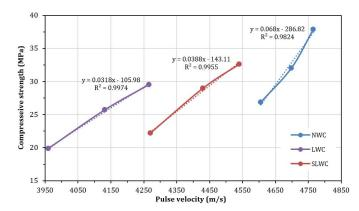
Fig. 6 Compressive strength vs pulse velocity after 28 days of curing
