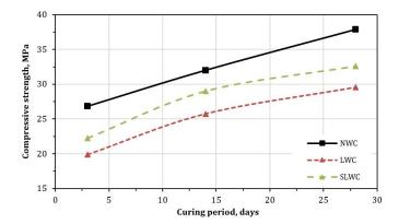
Fig. 4 Compressive strength development in SLWC and LWC specimens
