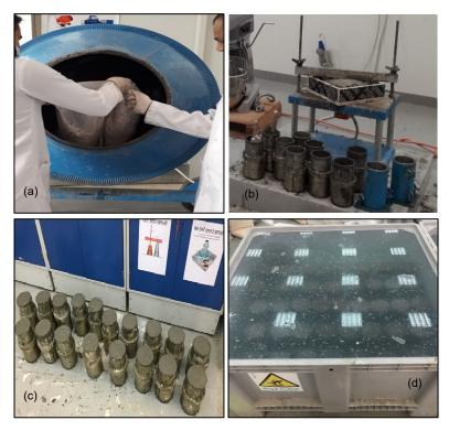
Fig. 3 Concrete casting view: (a) mixing; (b) compaction; (c) finished specimens; (d) curing under water tank
