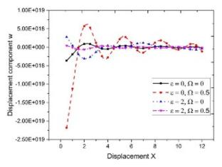
Fig. 5 Variation of displacement component *w* with displacement x at  $\Theta = 45^{\circ}$
