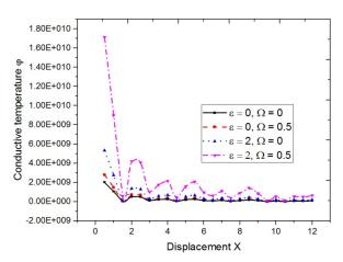
Fig. 12 Variation of conductive temperature  $\varphi$  with displacement x at  $\Theta = 30^{\circ}$
