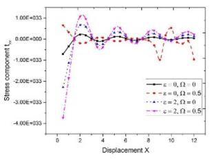
Fig. 11 Variation of stress component  $t_{xx}$  with displacement x at  $\Theta = 45^{\circ}$
