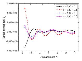
Fig. 6 Variation of stress component  $t_{zz}$  with displacement x at  $\Theta = 30^{\circ}$
