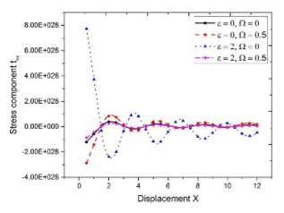
Fig. 10 Variation of stress component  $t_{xx}$  with displacement x at  $\Theta = 30^{\circ}$
