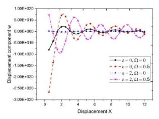
Fig. 4 Variation of displacement component w with displacement x at  $\Theta = 30^{\circ}$
