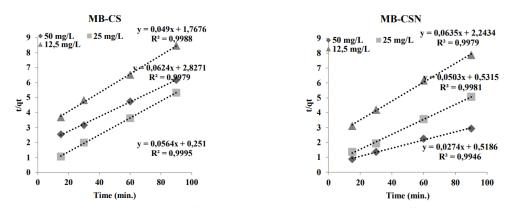
Fig. 10 Pseudo-second-order reaction for MB adsorbed onto CS and CSN at different concentrations
