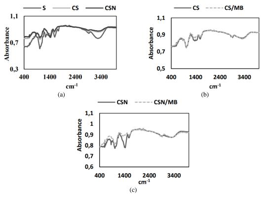
Fig. 4 FT-IR graphs of S, CS, CSN (a), CS and CS-MB (b), CSN and CSN-MB (c)
