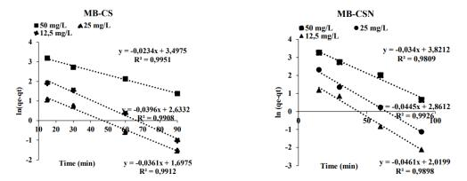
Fig. 9 Pseudo-first-order reaction for MB adsorbed onto CS and CSN at different concentrations
