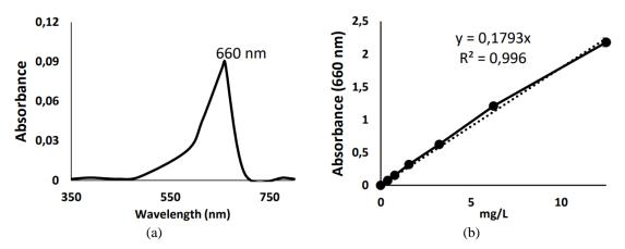
Fig. 1 (a) Wavelength scan of methylene blue dye at a concentration of 5 mg/L and (b) Standard chart for methylene blue dye at a concentration range of 0.39-12.5 mg/L
