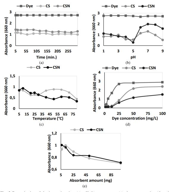
Fig. 2 Determination of the interaction time (a), pH (b), temperature (c), dye concentration (d) and adsorbent amount (e) for CS and CSN for methylene blue dye
