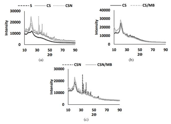
Fig. 5 XRD graphs of S, CS, CSN (a), CS, CS-MB (b) and CSN-MB(c)
