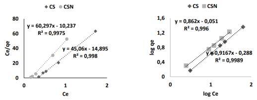
Fig. 8 Adsorption isotherms for the adsorption of MB onto CS and CSN. The inserts: the values of  $lnQ_e$  against  $lnC_e$  based on the Freundlich isotherm model and the linear dependence of  $C_e/Q_e$  on  $C_e$  based on the Langmuir isotherm model
