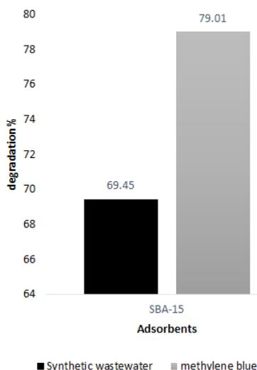
Fig. 14 Removing of the methylene blue comparison in optimum conditions (adsorbent of 200 mg/l, pH of 10, initial dye concentration of 20 mg/l and contact time 120 min) by MB pure and solution of MB in pH=10 and many component include many heavy metal and  $\text{Na}_2\text{S}_2\text{O}_4$
