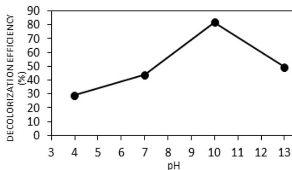
Fig. 6 The effect of pH in the removal rate of methylene blue
