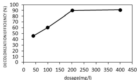
Fig. 7 Amount of adsorbent on the removal of methylene blue
