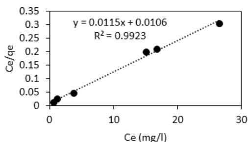
Fig. 13 Langmuir adsorption models of methylene blue on the SBA-15
