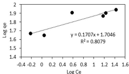
Fig. 12 Freundlich adsorption models of methylene blue on the SBA-15
