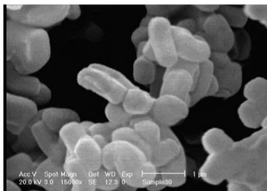
Fig. 5 SEM image calcined of hexagonal SBA-15 (the magnification $\times$ 15000)
