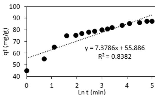
Fig. 9 Ellovich adsorption models of methylene blue on the SBA-15
