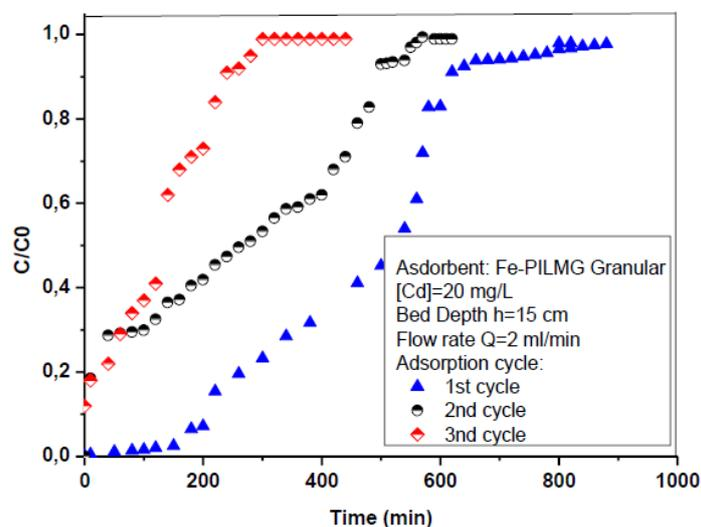
Fig. 6 Adsorption cycles of Fe-PILMG after three successive regenerations cycles
