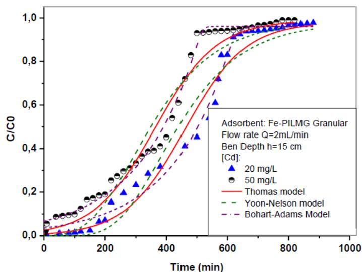
Fig. 4 Effect of Cd(II) concentration on the breakthrough curve adsorption on Fe-PILMG
