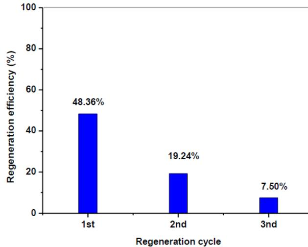
Fig. 7 Regeneration efficiency of Fe-PILMG granules after each regeneration cycle
