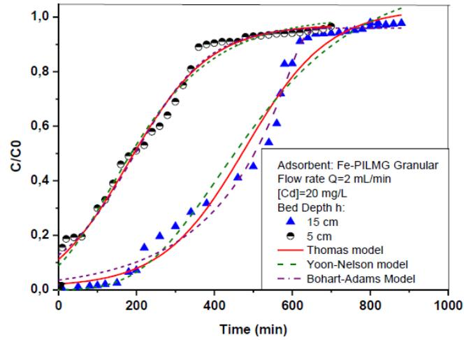
Fig. 2 Effect of various bed depths on the breakthrough curve of Cd(II) adsorption on Fe-PILMG
