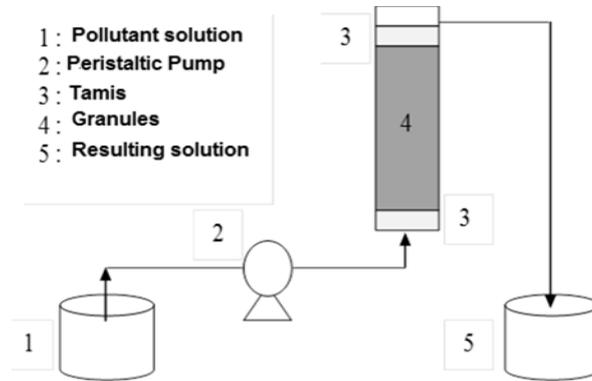
Fig. 1 Experimental method used in the dynamic adsorption of Cd(II) on a fixed bed based on Fe-PLIMG granules
