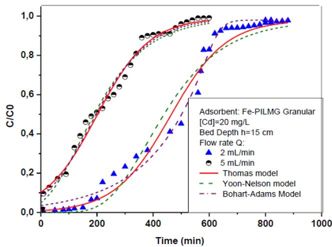
Fig. 3 Effect of flow rate on dynamic adsorption of Cd(II) on Fe-PILMG granules
