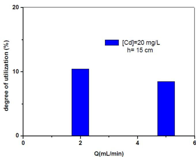
Fig. 5 Degree of utilization of Fe-PILMG granules bed
