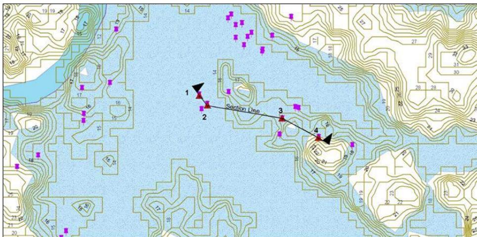
Fig. 1 Selected survey points and section line for cross-section to show temporal flood levels
