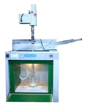
Fig. 1 Modified microwave heating system used for transesterification reactions
