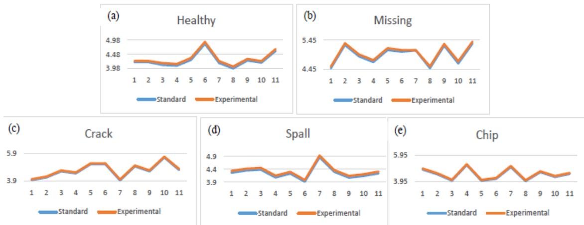
Fig. 6 Crest Factor Feature Vector under varied conditions; (a) Healthy, (b) Missing teeth, (c) Crack, (d) Spall and (e) Chip
