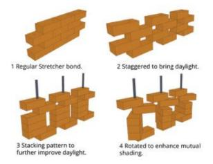
(a) Rotated patterns of outer skin for enhanced shading and improved daylight
