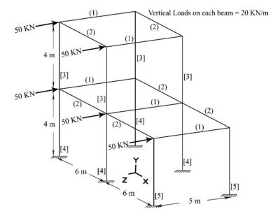
Fig. 13 Two-Story, Two bay irregular steel space frame
