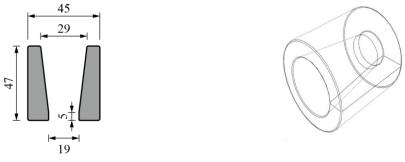
Fig. 1 Initial model of the tubular body (unit: mm)
