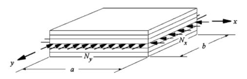
Fig. 1 A symmetric laminate under compressive biaxial loads
