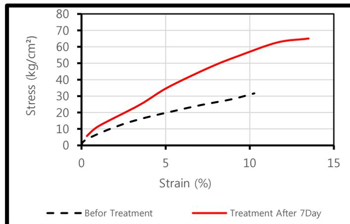
Fig. 5 Unconfined compression strength curves Before and After Treatment 7 days
