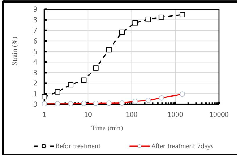
Fig. 6 Swelling Potential curves Before and After Treatment 7 days
