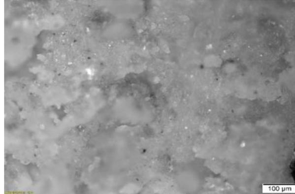
Fig. 8b Scanning electron micrograph of treatment lime 6% after 7days
