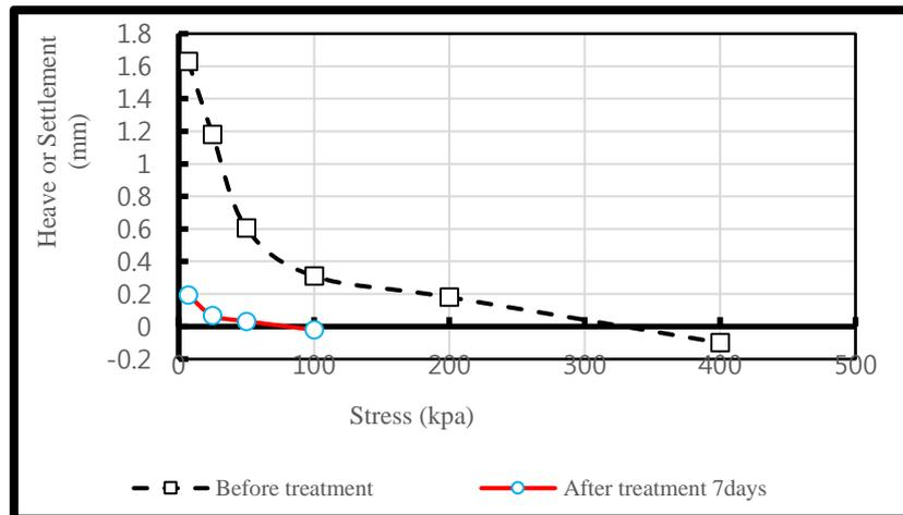
Fig. 7 Swelling Pressure curves before and after Treatment 7 days
