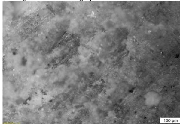
Fig. 8c Scanning electron micrograph of treatment lime 6% after 28 days
