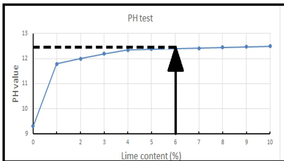
Fig. 2 Relationship between pH values and Lime content (%) to determine the optimum lime content of an expansive shell
