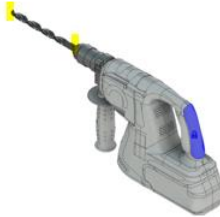
Fig. 3 Drill with highlighted stress points
