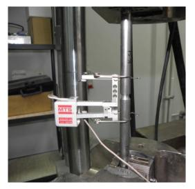
Fig. 3 An exemplary notched specimen under static tension
