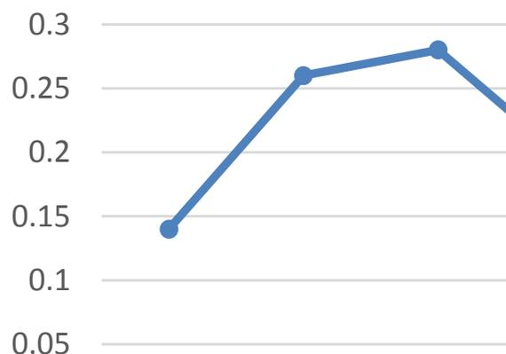
Fig. 1 Collapse probability under the condition of different tunnel buried depth
