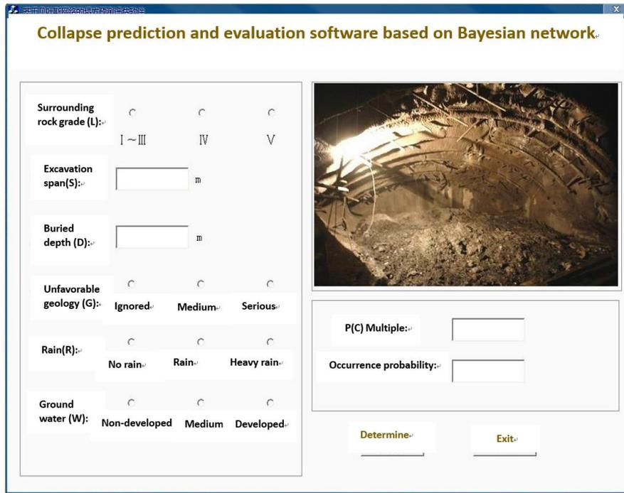
Fig. 5 Collapse prediction software based on Bayesian network
