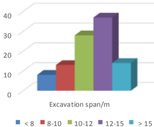
Fig. 3 Collapse probability under the condition of different excavation span
