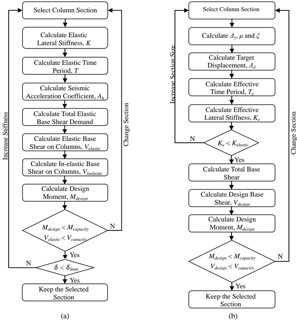
Fig. 4 Flow chart of (a) FBD and (b) DDBD Methodology
