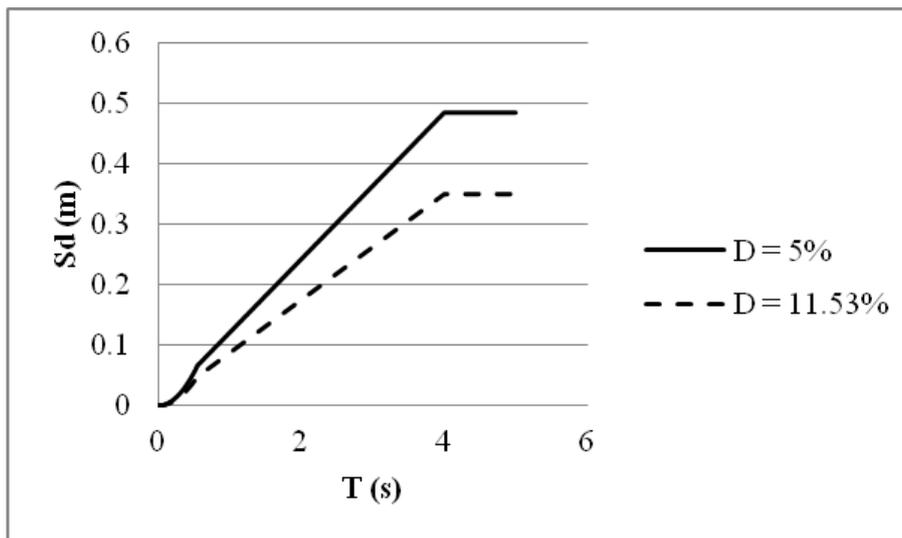
Fig. 6 Displacement response spectra
