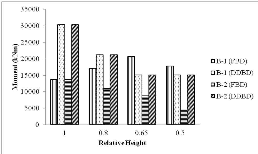
Fig. 8 Variation of moment at bents with design methodology
