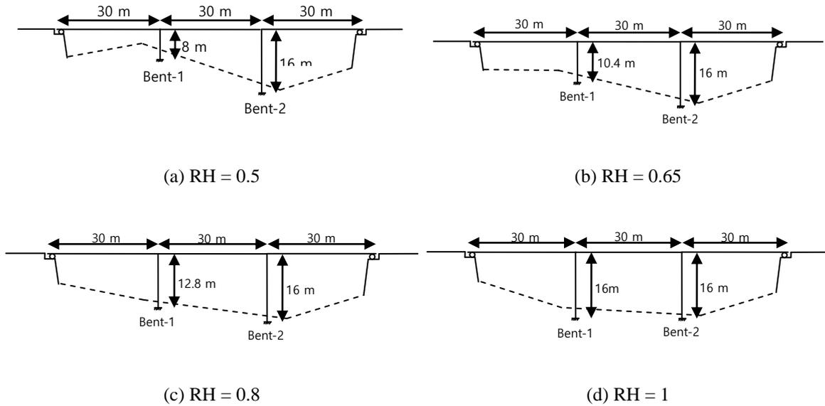
Fig. 3 Bridge geometry used in the study of seismic irregularity
