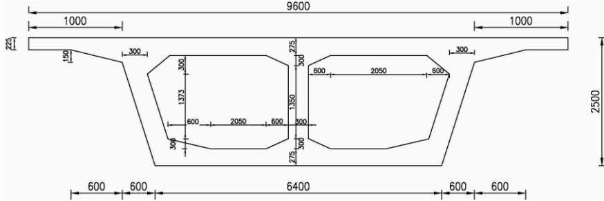
Fig. 2 Geometry and dimension detail of the deck (all dimensions in mm)
